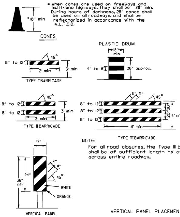
NOTE: For all road closures, the Type III barricades shall be of sufficient length to extend across entire roadway.
