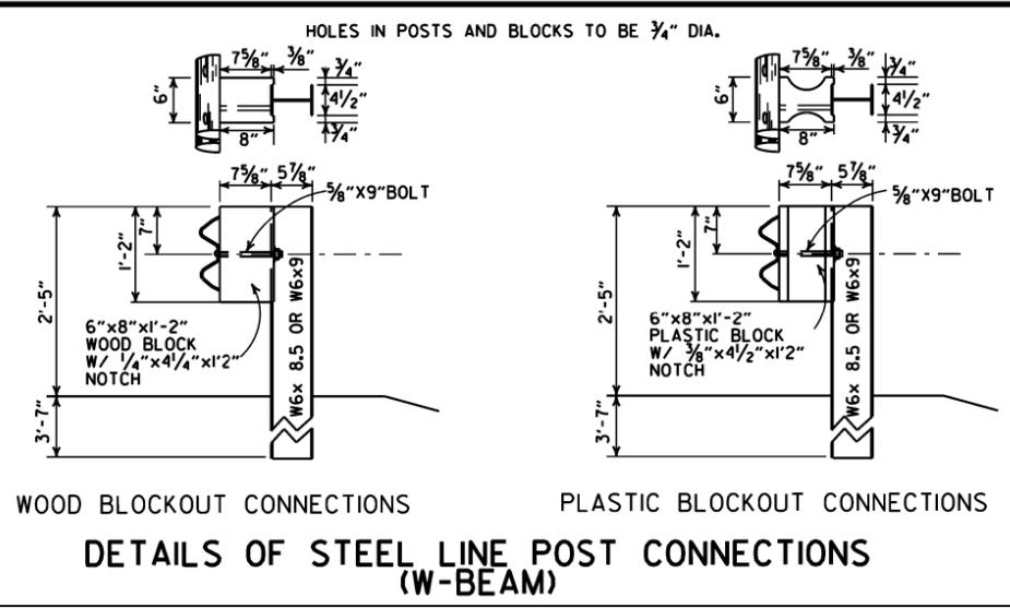
**WOOD BLOCKOUT CONNECTIONS
