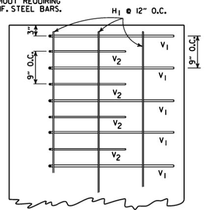
**PLAN OF REINFORCING STEEL IN FOOTING**
