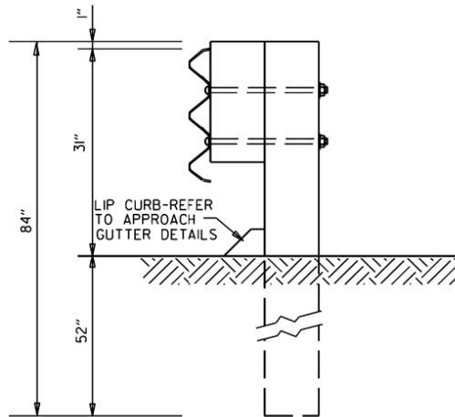
THRIE BEAM RAIL WITH WOOD OR PLASTIC BLOCKOUTS & WOOD POSTS
