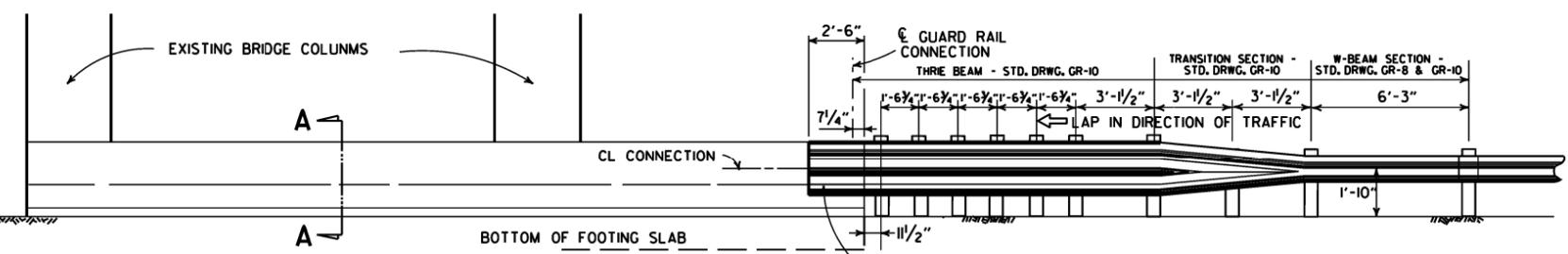
NOTE: ALL EXPOSED EDGES OF THE CONCRETE BARRIER WALL SHALL HAVE A 3/4" CHAMFER.
