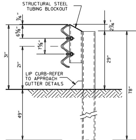
THRIE BEAM RAIL WITH STEEL TUBING BLOCKOUT AND STEEL POST
