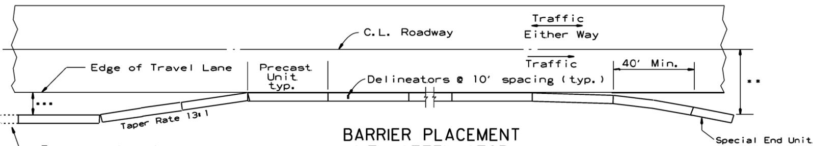
**BARRIER PLACEMENT WITH ATTENUATOR**
