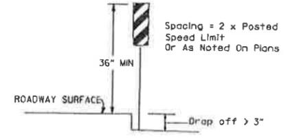
TRAFFIC CONTROL DEVICES FOR VERTICAL PAVEMENT DIFFERENTIALS
