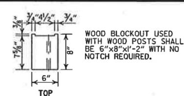
WOOD BLOCKOUT USED WITH WOOD POSTS SHALL BE 6"X8"X1'-2" WITH NO NOTCH REQUIRED.
