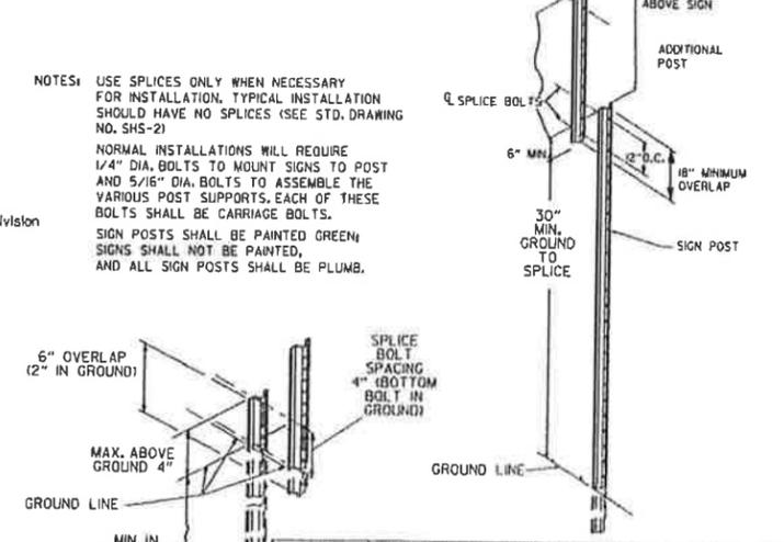
NOTES: USE SPLICES ONLY WHEN NECESSARY FOR INSTALLATION. TYPICAL INSTALLATION SHOULD HAVE NO SPLICES (SEE STD. DRAWING NO. SHS-2). NORMAL INSTALLATIONS WILL REQUIRE 1/4" DIA. BOLTS TO MOUNT SIGNS TO POST AND 5/16" DIA. BOLTS TO ASSEMBLE THE VARIOUS POST SUPPORTS. EACH OF THESE BOLTS SHALL BE CARRIAGE BOLTS. SIGN POSTS SHALL BE PAINTED GREEN; SIGNS SHALL NOT BE PAINTED, AND ALL SIGN POSTS SHALL BE PLUMB.
