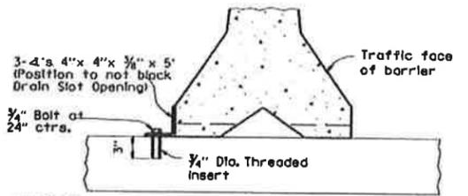
NOTE: 3/4" Threaded Inserts shall be cast in place for all new bridge decks and drilled and grouted for existing bridge decks. Inserts shall have a minimum ultimate load capacity of 8000 lbs. in tension. After removal of barrier, bolts, and angles, the inserts shall be filled with approved non-shrink epoxy.
