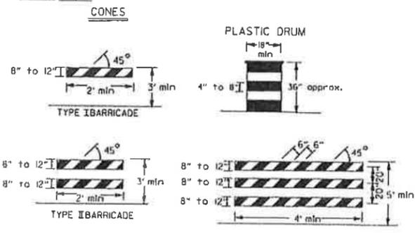
NOTE: For all road closures, the Type III barricades shall be of sufficient length to extend across entire roadway.
