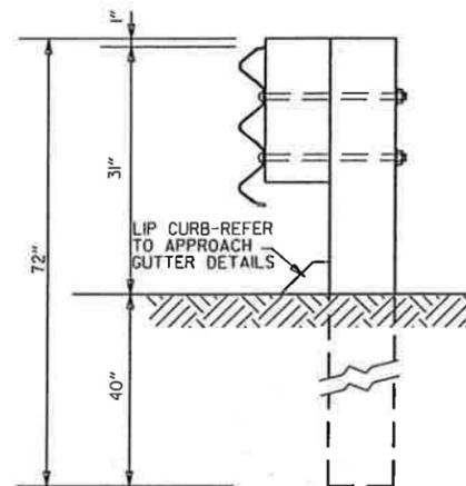
THRIE BEAM RAIL WITH WOOD OR PLASTIC BLOCKOUT & WOOD POST
