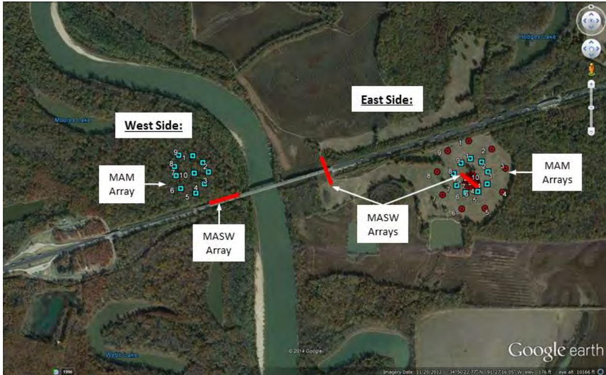
Figure 1. Current I-40 bridge over the White River (location 34.83967° N 91.4572° W). Also shown are the locations of the sensor arrays used for active-source multi-channel analysis of surface waves (MASW) testing and ambient-wavefield microtremor array measurements (MAM) on the West and East sides of the river.
