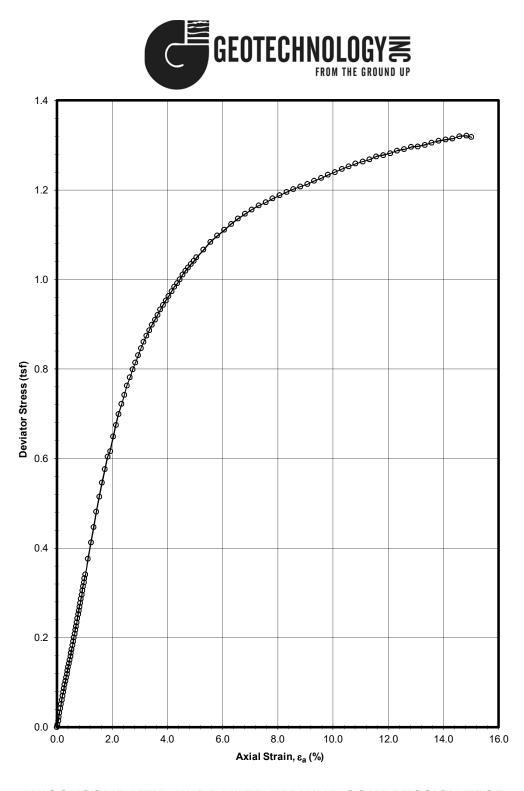
UNCONSOLIDATED-UNDRAINED TRIAXIAL COMPRESSION TEST ASTM D 2850 Project No.: J034363.01 Boring: VC-3 Sample: ST-12 - Depth: 43 ft.
