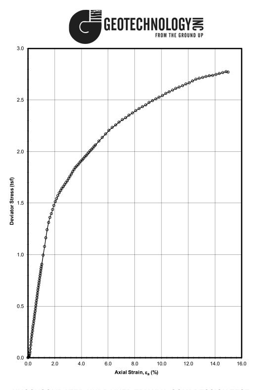
UNCONSOLIDATED-UNDRAINED TRIAXIAL COMPRESSION TEST ASTM D 2850 Project No.: J034363.01 Boring: VC-1 Sample: ST-11 - Depth: 33 ft.
