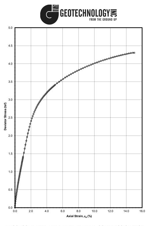
UNCONSOLIDATED-UNDRAINED TRIAXIAL COMPRESSION TEST ASTM D 2850 Project No.: Boring: VC-3 Sample: ST-17 - Depth: 60 ft.
