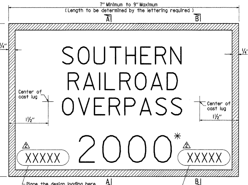
TYPICAL BRIDGE NAME PLATE-STYLE 3 - FULL SIZE GRADE SEPARATION STRUCTURES
