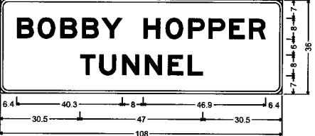
ML49-45-3NB ; 3.0" Radius, 1.0" Border, White on Green; [BOBBY HOPPER] E Mod 2K; [TUNNEL] E Mod 2K;
