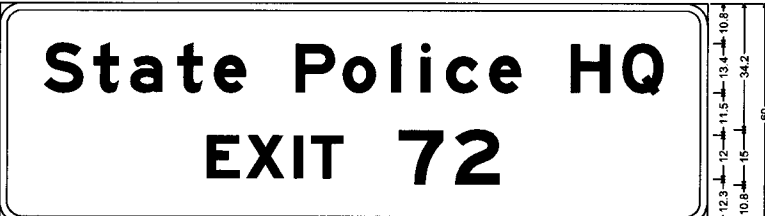
ML49-72-1SB ; 6.0" Radius, 2.0" Border, White on Blue; [State Police HQ] E Mod 2K; [EXIT] E Mod 2K; [72] E Mod 2K;
