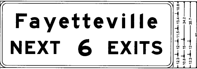
ML49-67-1SB ; 6.0" Radius, 2.0" Border, White on Green; [Fayetteville] E Mod 2K; [NEXT] E Mod 2K; [6] E Mod 2K; [EXITS] E Mod 2K;
