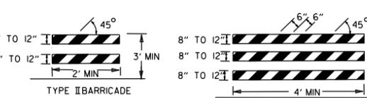
NOTE: FOR ALL ROAD CLOSURES, THE TYPE III BARRICADES SHALL BE OF SUFFICIENT LENGTH TO EXTEND ACROSS ENTIRE ROADWAY.
