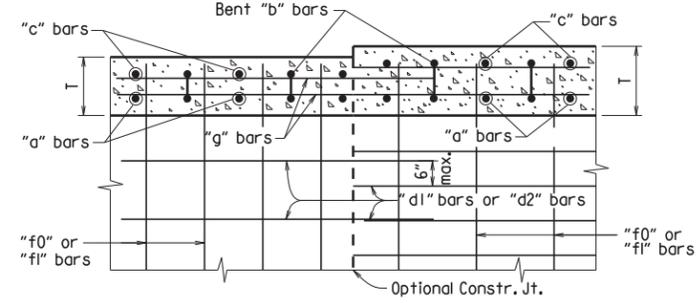
Longitudinal Bar Spacing at individual sections shall be maintained, which may result in noncontact bar laps.
