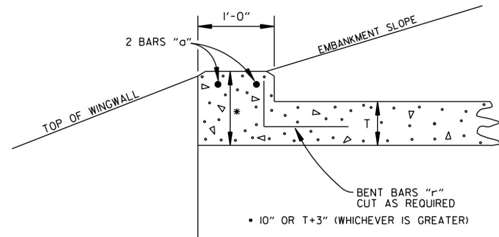
NOTE: FOR ALL SKEWED R.C. BOX CULVERTS THE LENGTH "K" OF THE MODIFIED HEADWALL SHALL BE EQUAL TO THE ROADWAY LENGTH "RL". THE ENDS OF THE HEADWALL SHALL BE CONSTRUCTED PARALLEL TO THE SKEW ANGLE OF THE BOX CULVERT.
