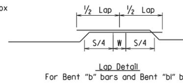
At the Contractor's option in lieu of providing Bent "b" or Bent "bl" bars, one bar top and bottom of equivalent size may be substituted for each bent bar. Payment for the reinforcing will be based on the weight of the "b" or "bl" bar.
