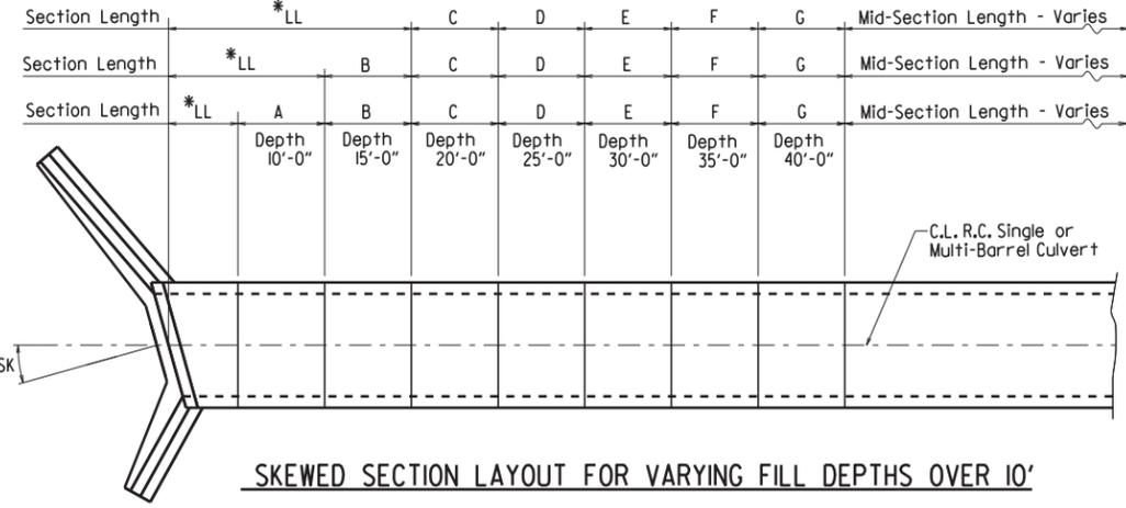
SKewed SECTION LAYOUT FOR VARYING FILL DEPTHS OVER 10'
