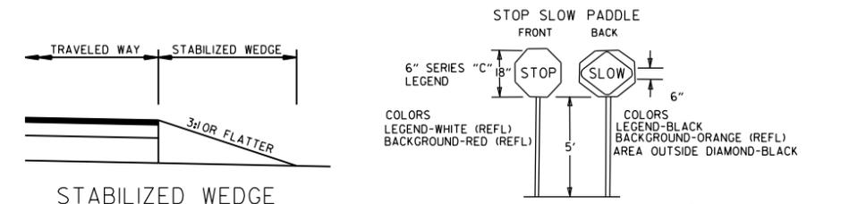
NOTE: MATERIALS FOR THE STABILIZED WEDGE SHALL MEET THE REQUIREMENTS PROVIDED IN SECTION 603.02 OF THE STANDARD SPECIFICATIONS.
