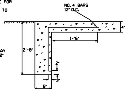
TOE WALL DEPTH MAY BE ALTERED TO 1'-0" WHEN DIRECTED BY THE ENGINEER IN ROCK EXCAVATION
