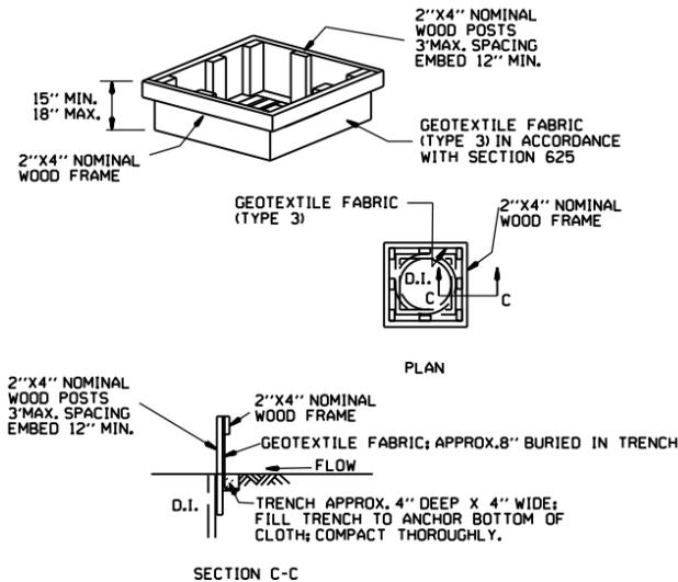
**DROP INLET SILTS FENCE (E-7)**
