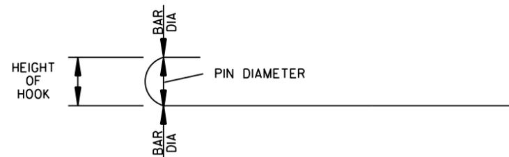
NOTE: DIMENSIONS OF BARS ARE MEASURED OUT TO OUT OF BARS.
