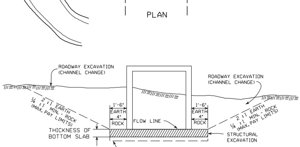
SECTION B-B DETAILS FOR NEW CHANNELS
