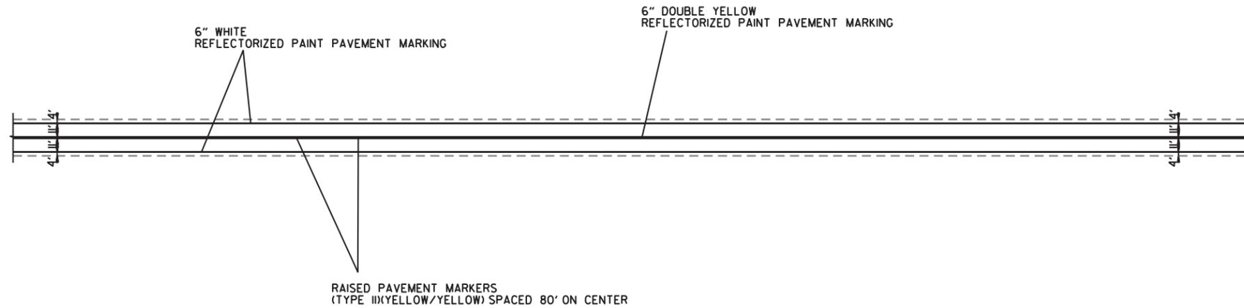
TYPICAL 2-LANE PERMANENT PAVEMENT MARKING LAYOUT
