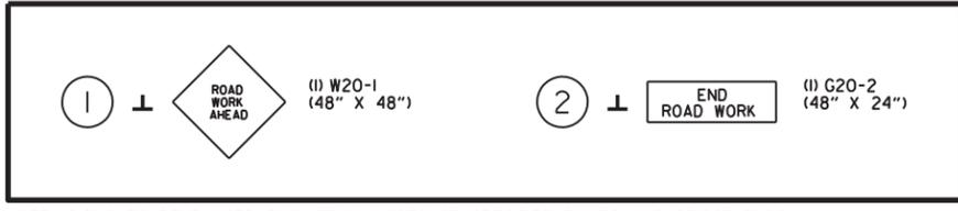
NOTE: SIGNS TO BE PLACED 500' FROM NOSES OF SPECIFIED RAMPS AND BRIDGE ENDS.
