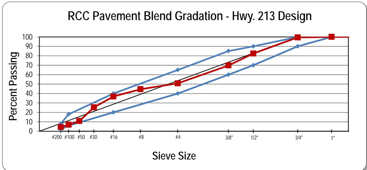
**Figure 13. RCC Gradation and Specification Band**
