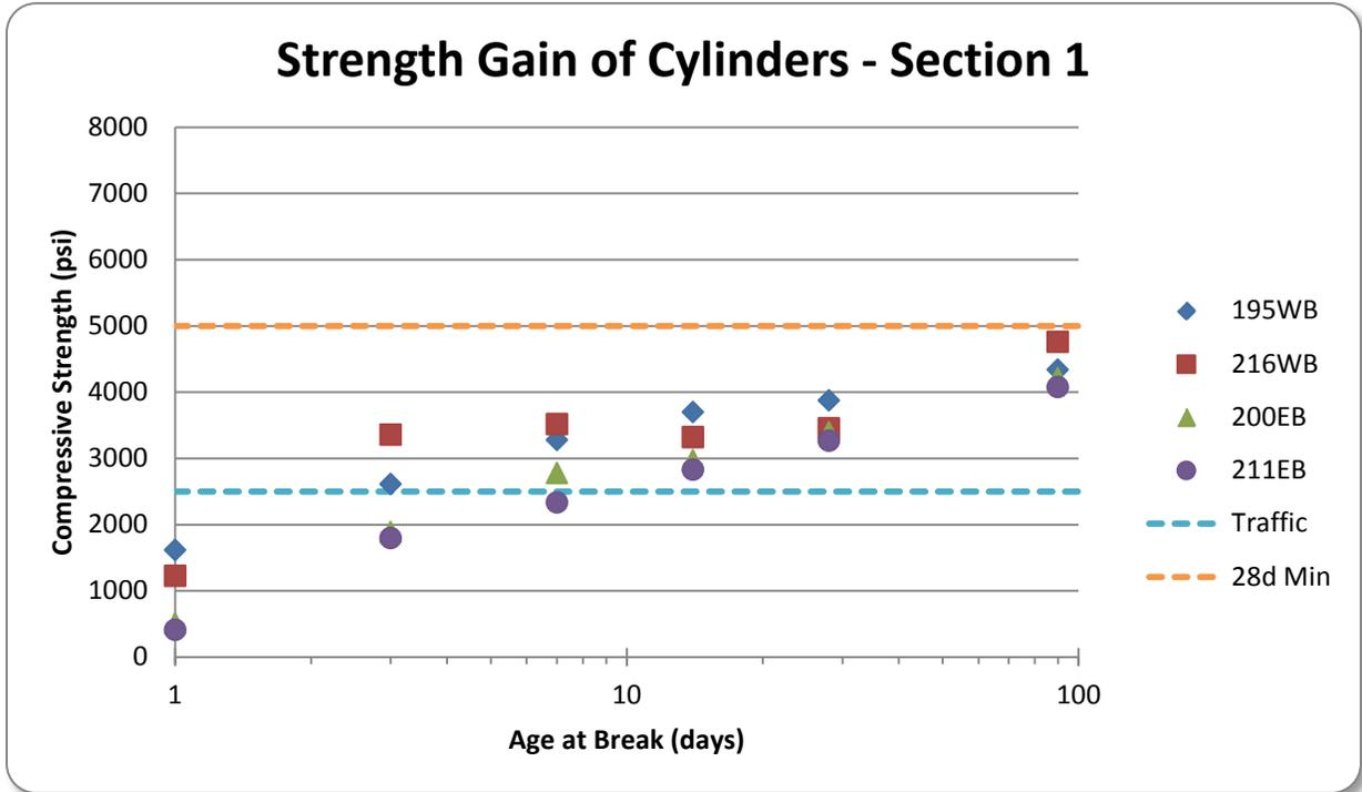
Figure 38. Compressive Strength of Cylinders Over Time – Section 1
