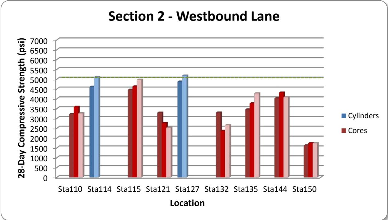
Figure 46. Compressive Strength Comparison of Cylinders and Cores – Section 2 WB
