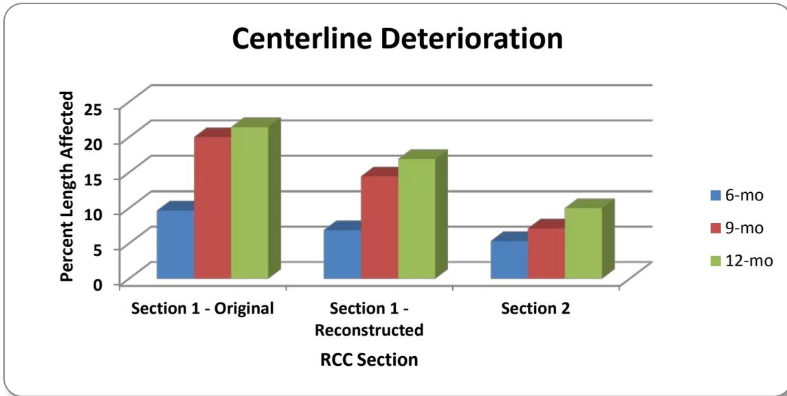
**Figure 66. Centerline Deterioration by Section**
