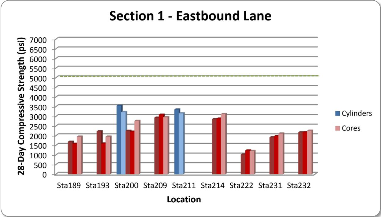
Figure 45. Compressive Strength Comparison of Cylinders and Cores – Section 1 EB
