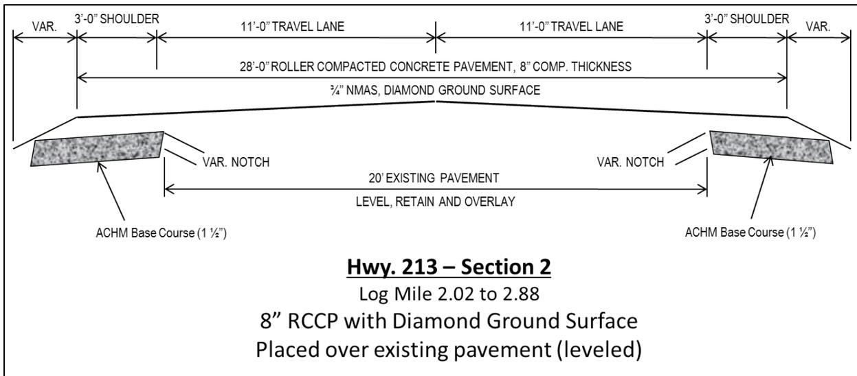
**Figure 12. Typical Sections for RCC Construction**
