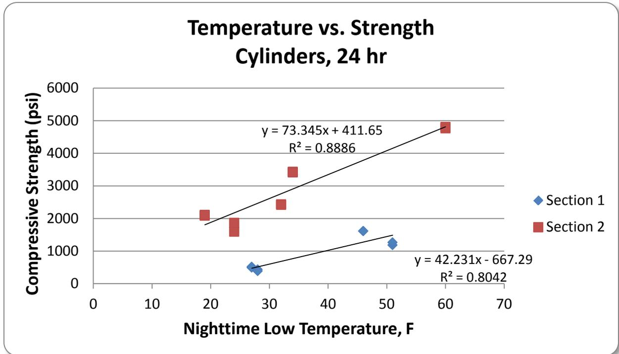
**Figure 50. Low Temperature vs. Compressive Strength at 24 hours**
