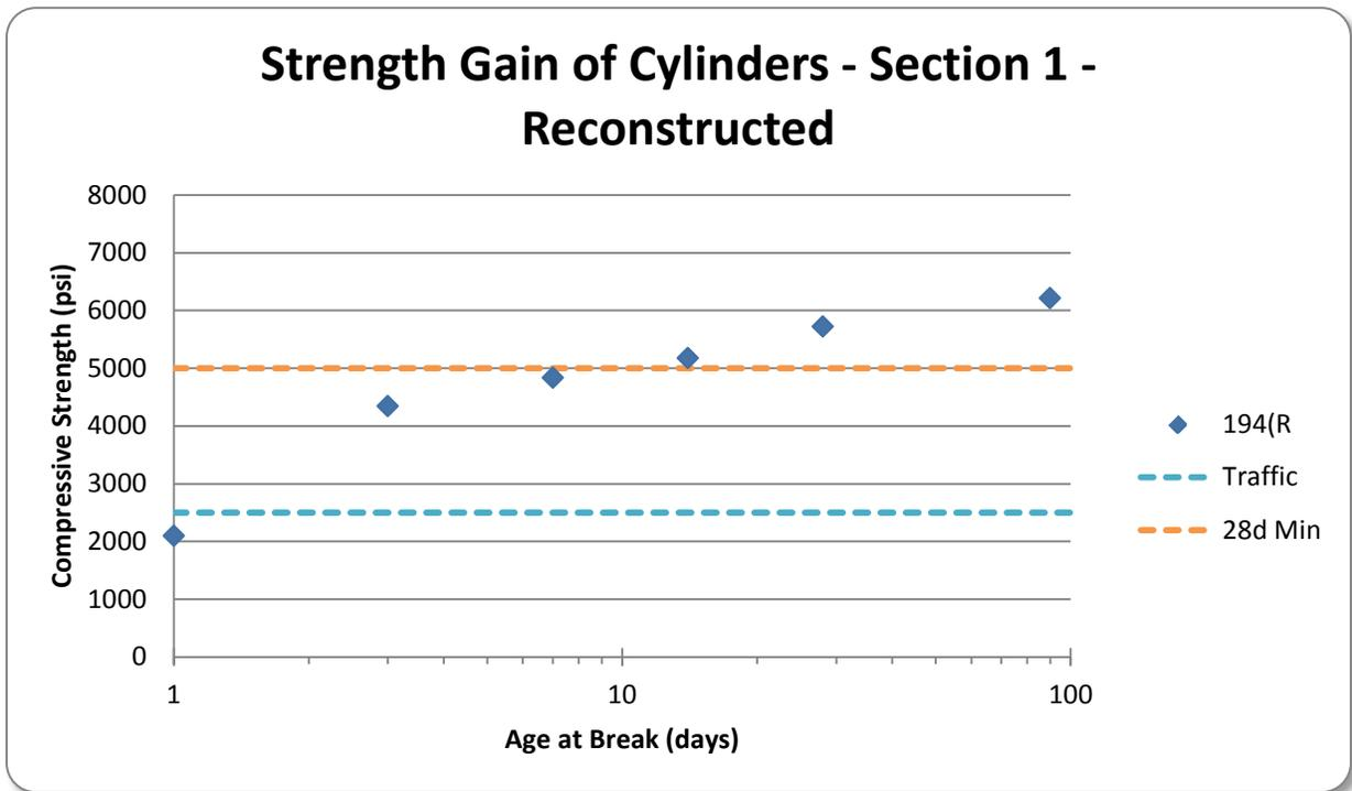
**Figure 43. Compressive Strength of Cylinders Over Time – Section 1 (Reconstructed)**
