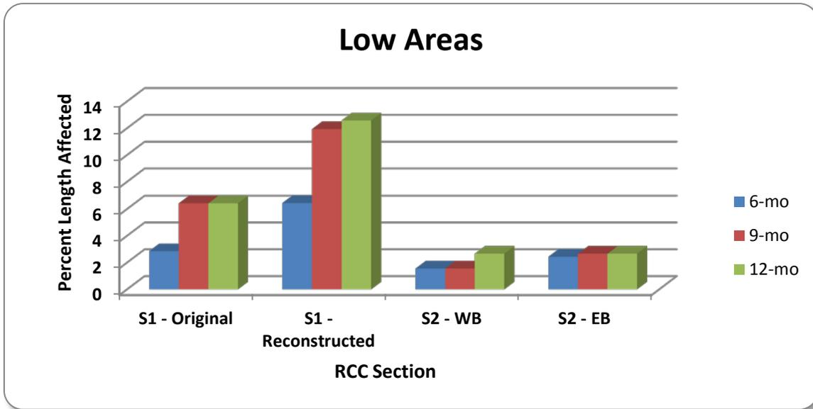
**Figure 90. Low Areas Visible by Section**
