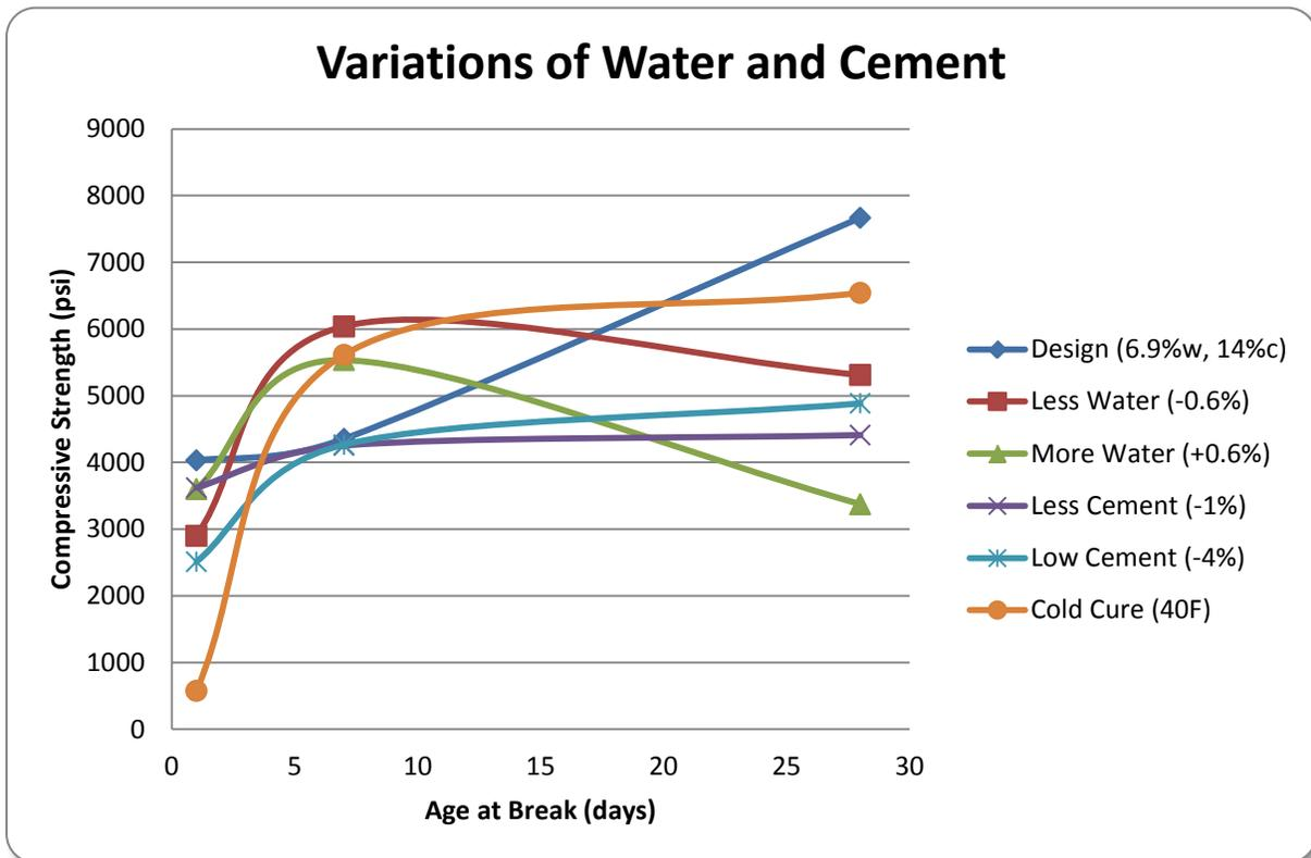
Figure 51. Comparison of Compressive Strength for Variations in Water Content, Cement Content, and Curing Temperature
