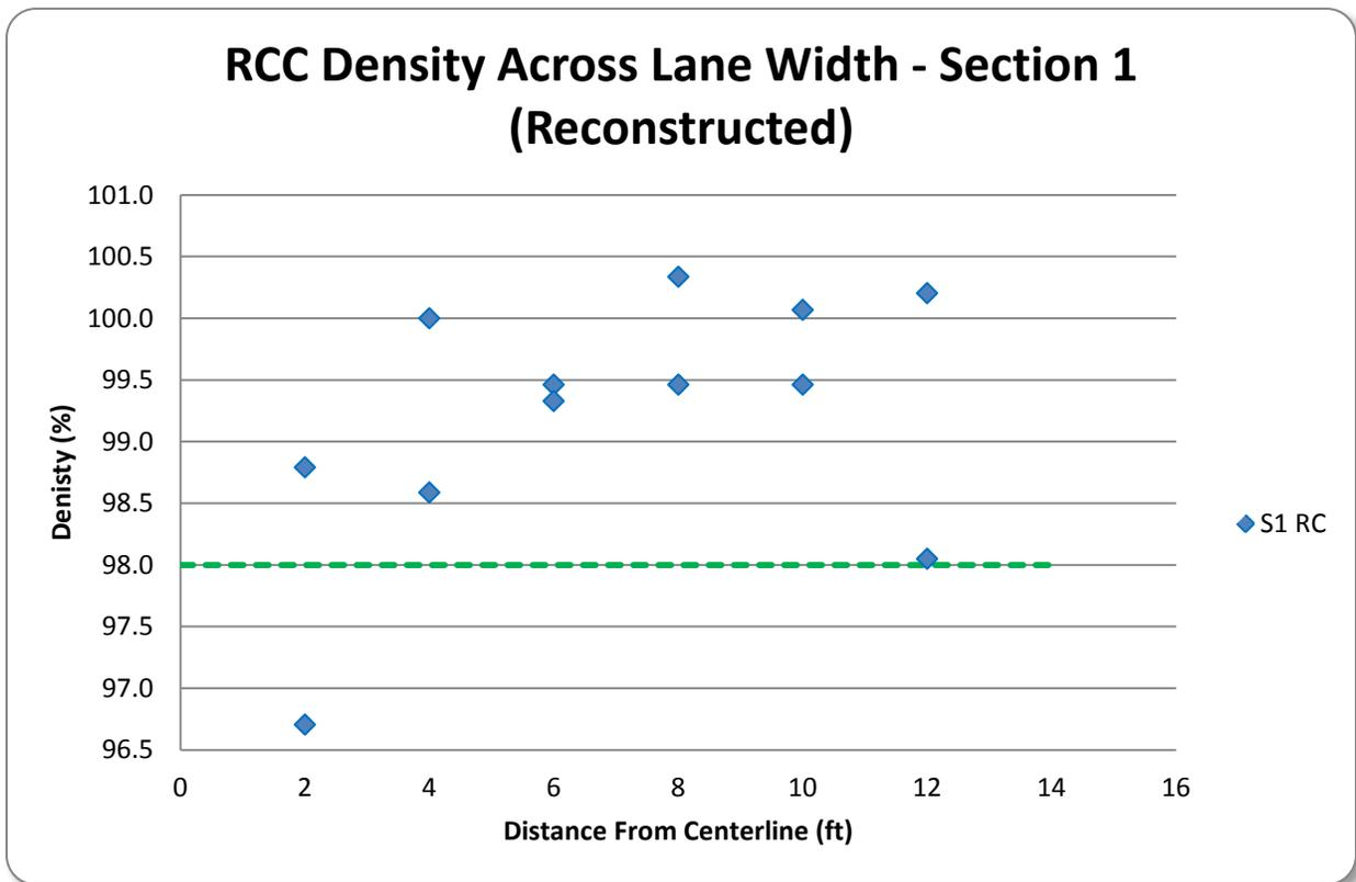
**Figure 42. RCC Density at Varying Distances from Centerline – Section 1 (Reconstructed)**
