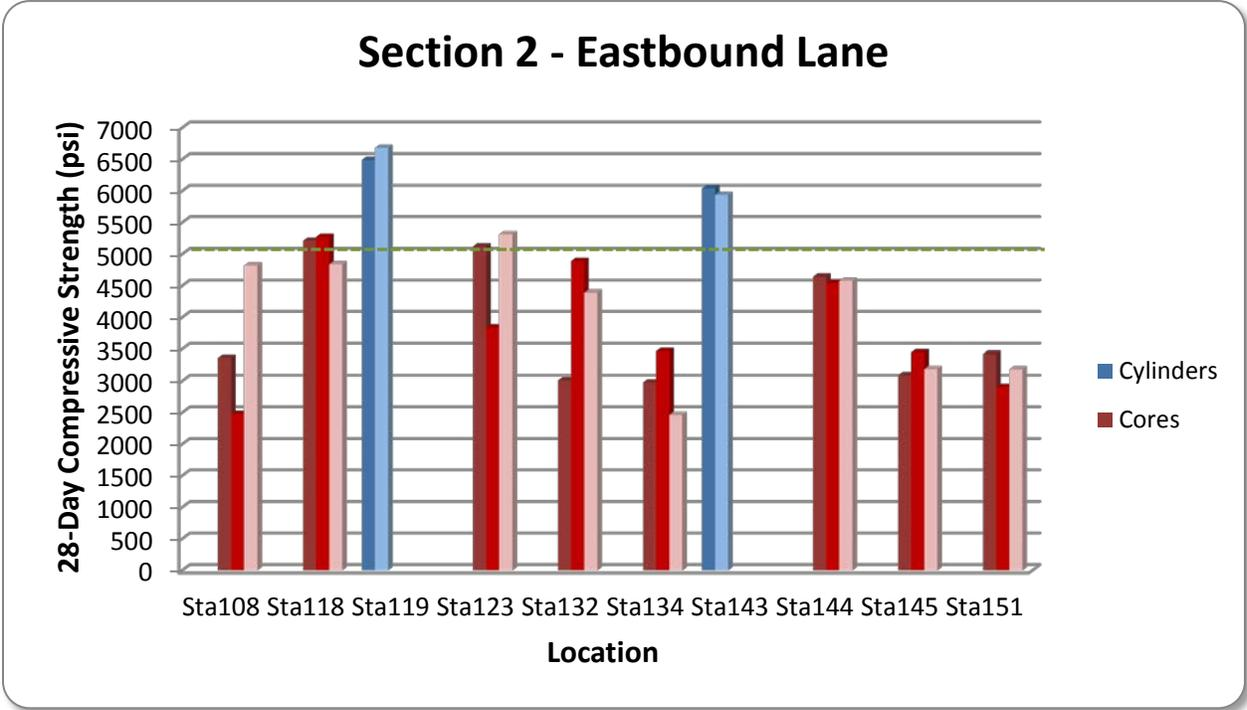
Figure 47. Compressive Strength Comparison of Cylinders and Cores – Section 2 EB
