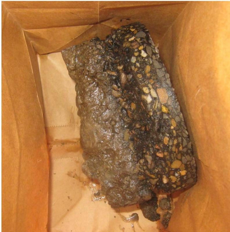
**Figure 11. Hwy. 213 Core of Minimal Asphalt Thickness**
