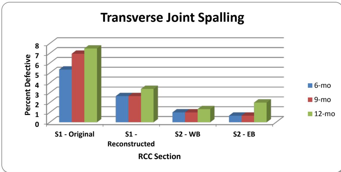
Figure 59. Transverse Joint Spalling by Section
