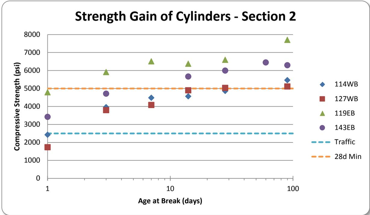
Figure 41. Compressive Strength of Cylinders Over Time – Section 2
