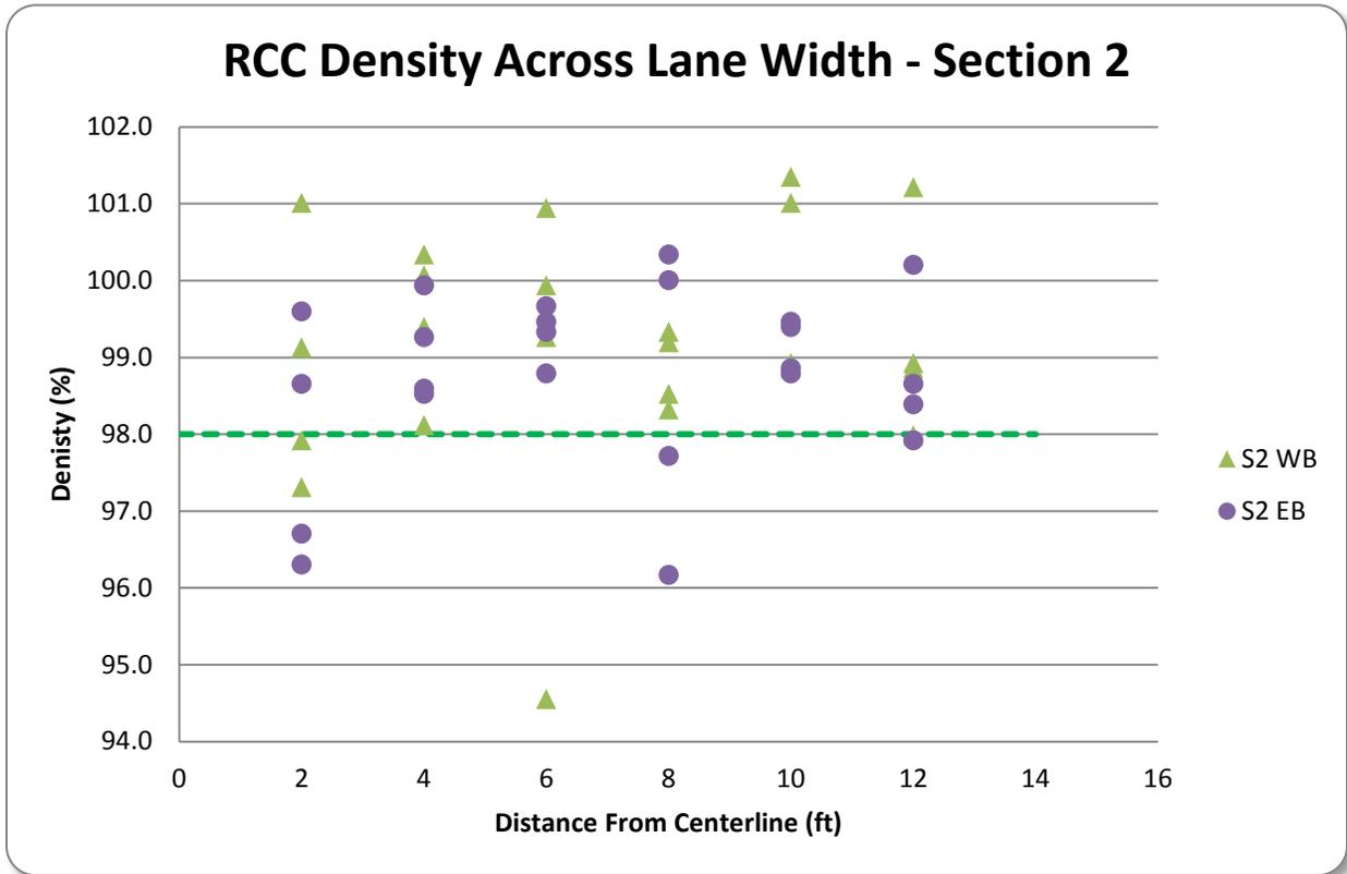
Figure 40. RCC Density at Varying Distances from Centerline – Section 2
