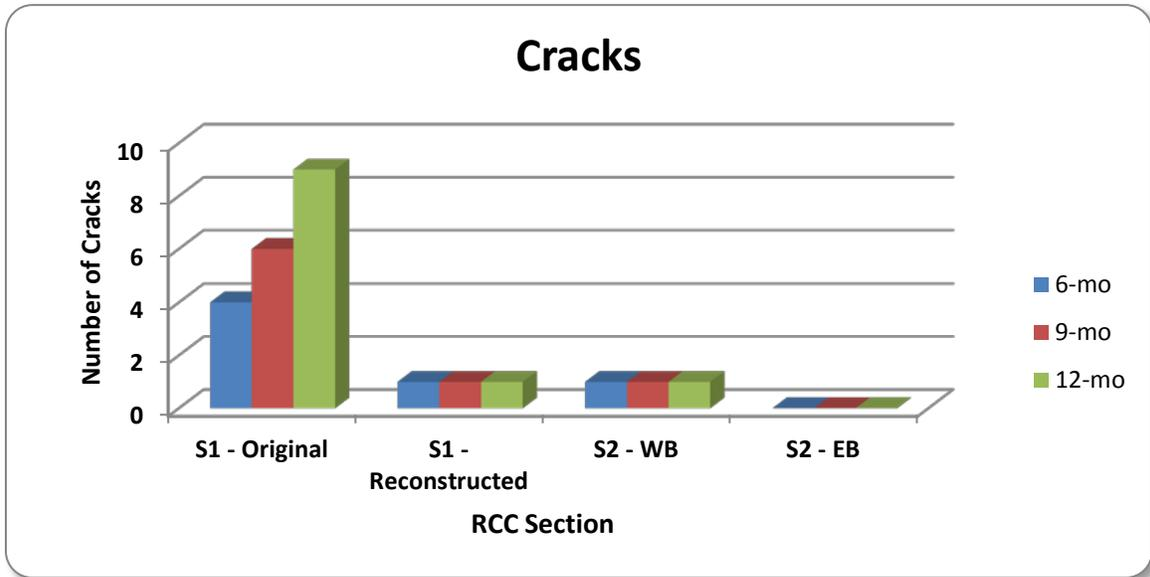
**Figure 71. Cracking Distress Summary by Section**
