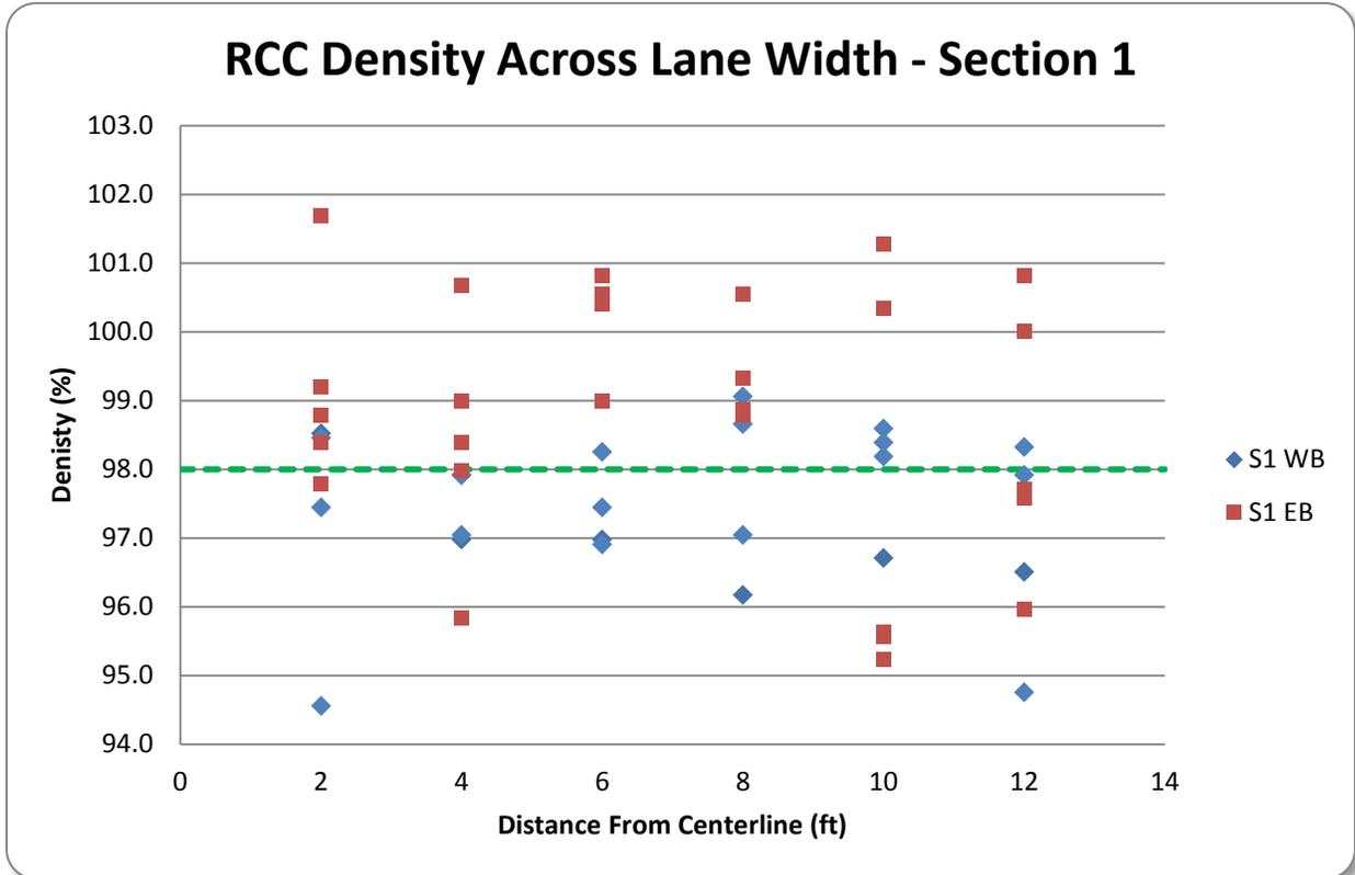
Figure 37. Density of RCC at Varying Distances from the Centerline – Section 1
