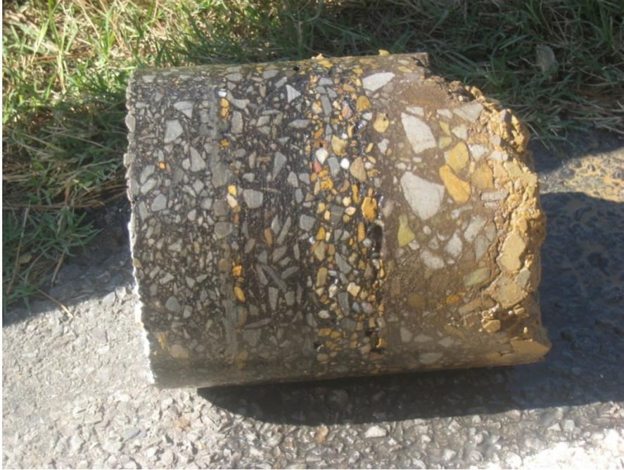
**Figure 10. Hwy. 213 Core with Several Layers**
