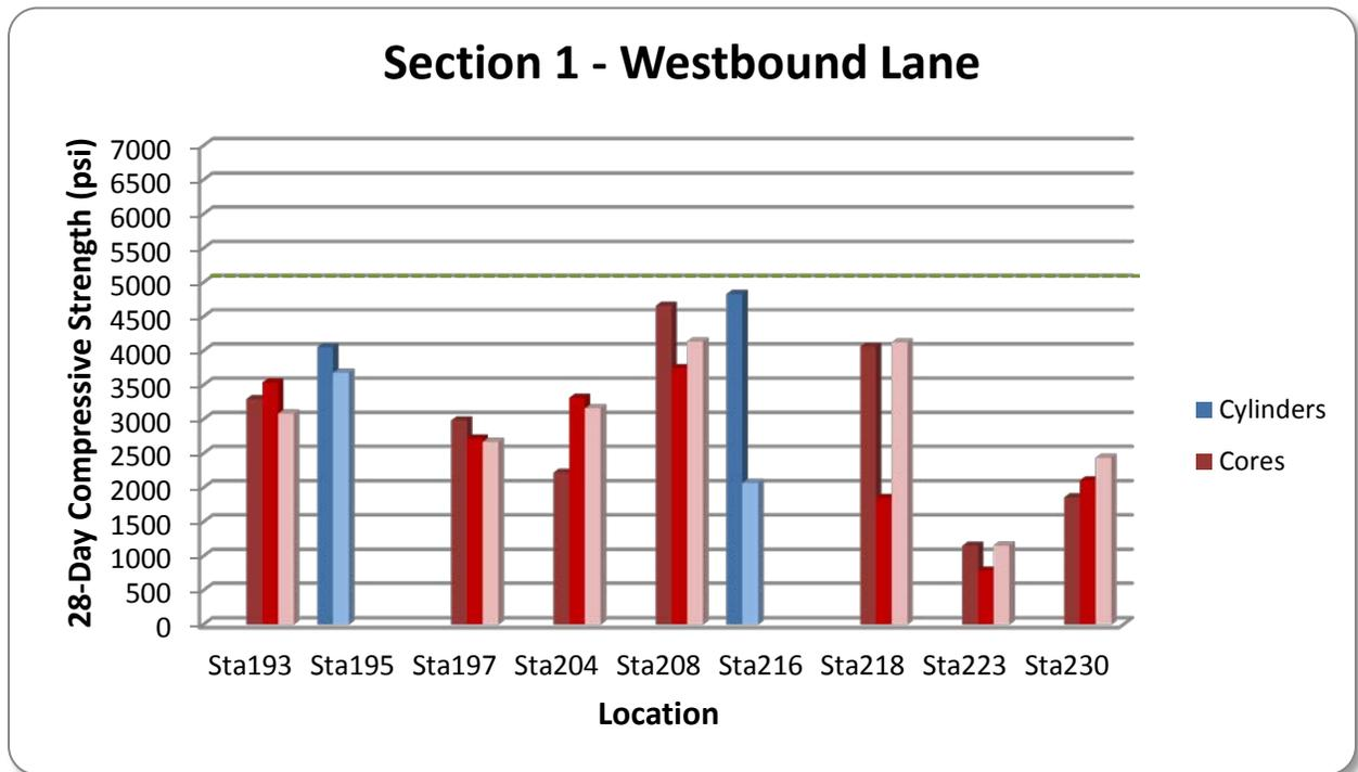
**Figure 44. Compressive Strength Comparison of Cylinders and Cores – Section 1 WB**
