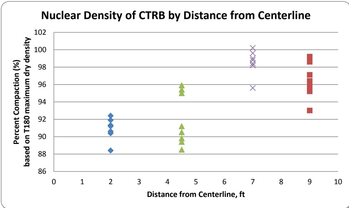
Figure 22. Density of CTRB in the Eastbound Lane for Varying Distances from the Centerline
