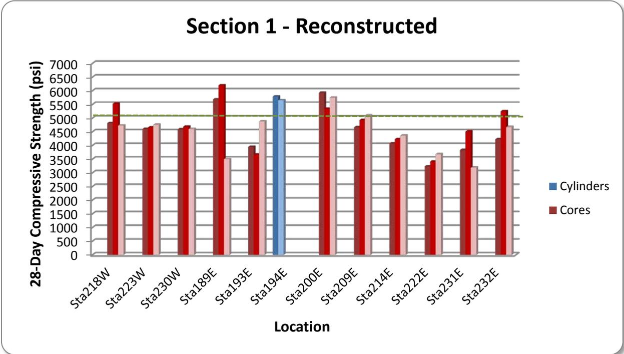
Figure 48. Compressive Strength Comparison of Cylinders and Cores – Section 1 - Reconstructed
