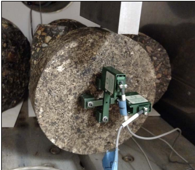
Figure 2.3 – Dynamic Modulus and Creep Compliance Testing Configuration (photo: Henrichs)
