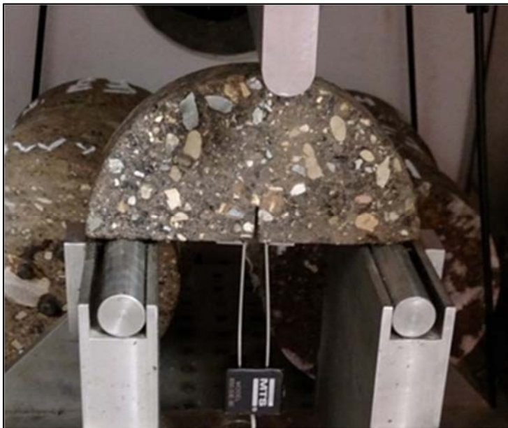
Figure 2.4 - Semi-Circular Bend Test Configuration (photo: Henrichs)
