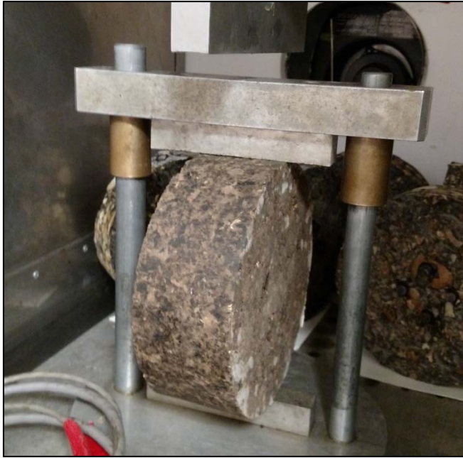
Figure 2.6 – Indirect Tensile Strength Test (photo: Henrichs)
