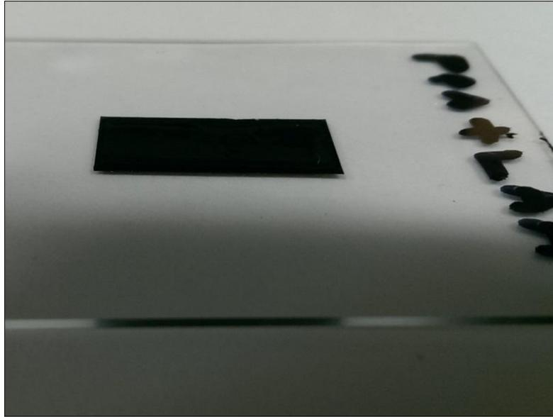
**Figure 4.21: An Asphalt Binder Sample Ready for OCA Test.**
