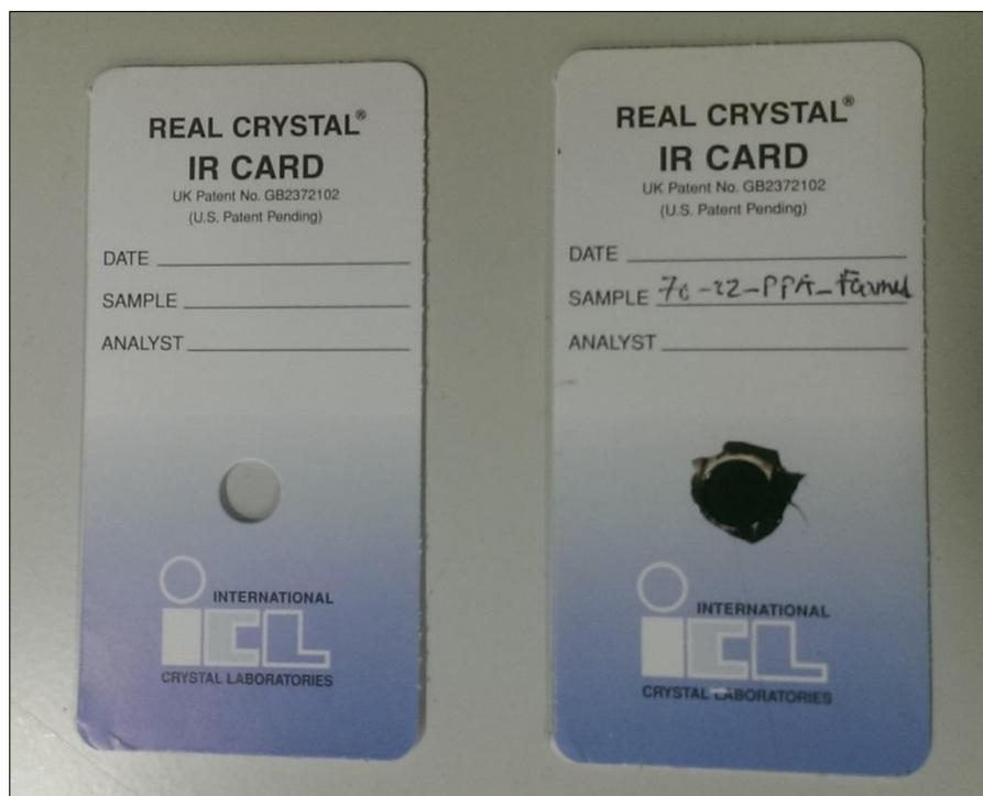
**Figure 4.18: An Empty IR card (Left) and a Sample Ready for FTIR Test (Right).**
