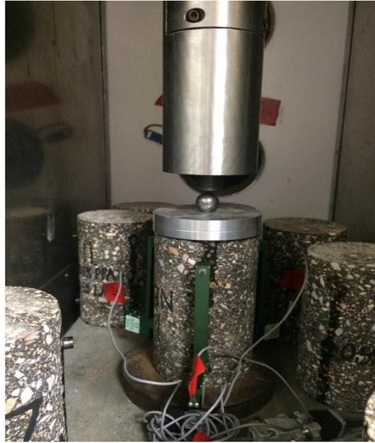
**Figure 4.25: Uniaxial Dynamic Modulus.**
