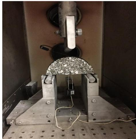
**Figure 4.26: SCB Test.**
