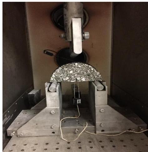
**Figure 4.26: SCB Test.**
