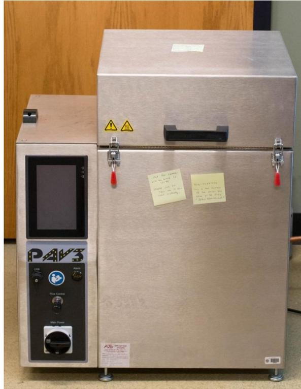
Figure 4.14: Pressure Aging Vessel (PAV).
