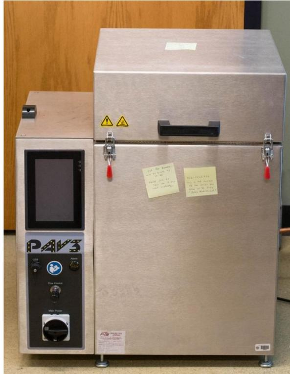
Figure 4.14: Pressure Aging Vessel (PAV).
