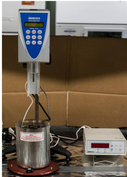
**Figure 4.10: RV Test Device.**
