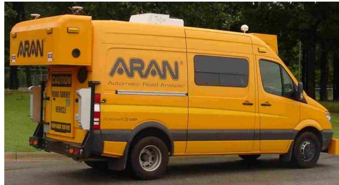
**Figure 4.27: Automated Road Analyzer**
