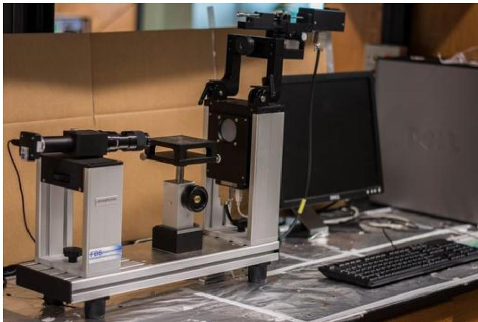
**Figure 4.20: Optical Contact Analyzer (OCA) Device.**
