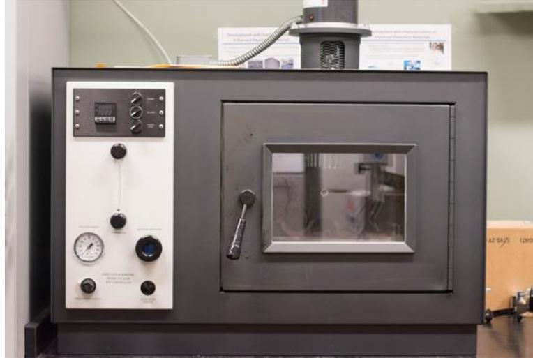
**Figure 4.13: Rotational Thin Film Oven (RTFO).**
