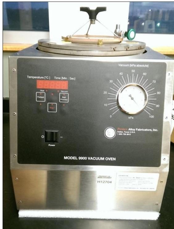
Figure 4.15: Vacuum Degassing Oven.
