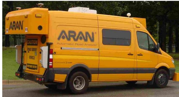
**Figure 4.27: Automated Road Analyzer**
