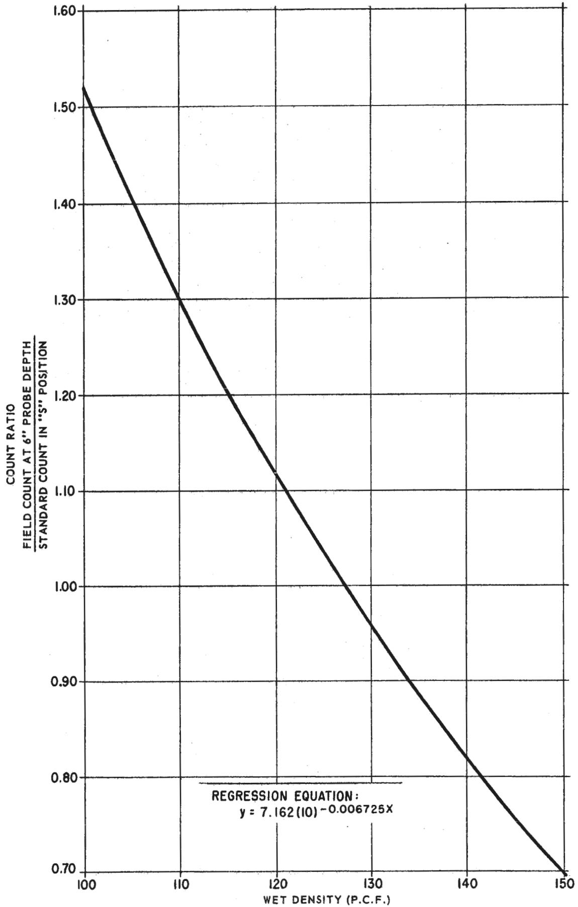
8" PROBE DEPTH CALIBRATION CURVE
