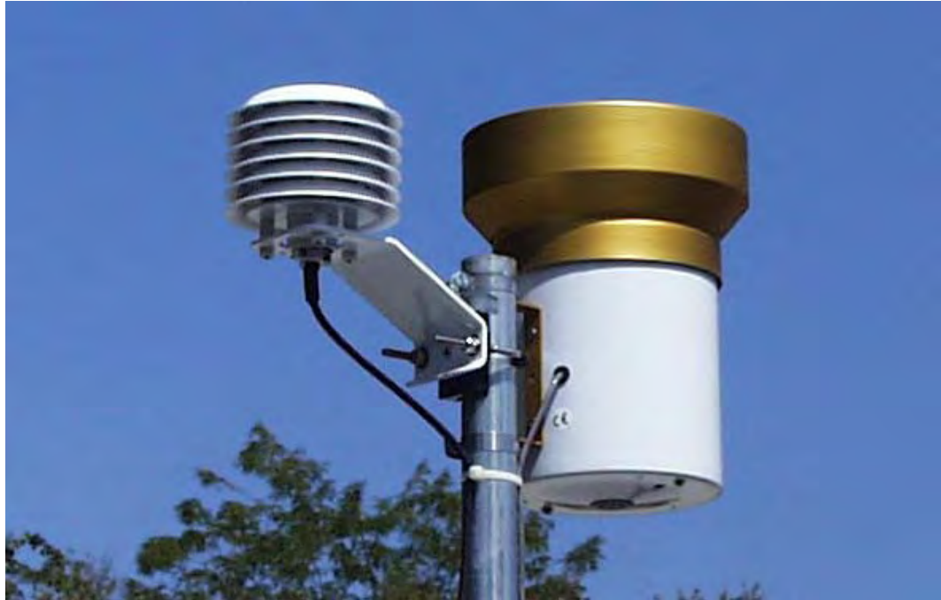
Figure 3.66 A 107 temperature probe (left), housed in a radiation shield, and a TR-525USW rainfall sensor (right).
