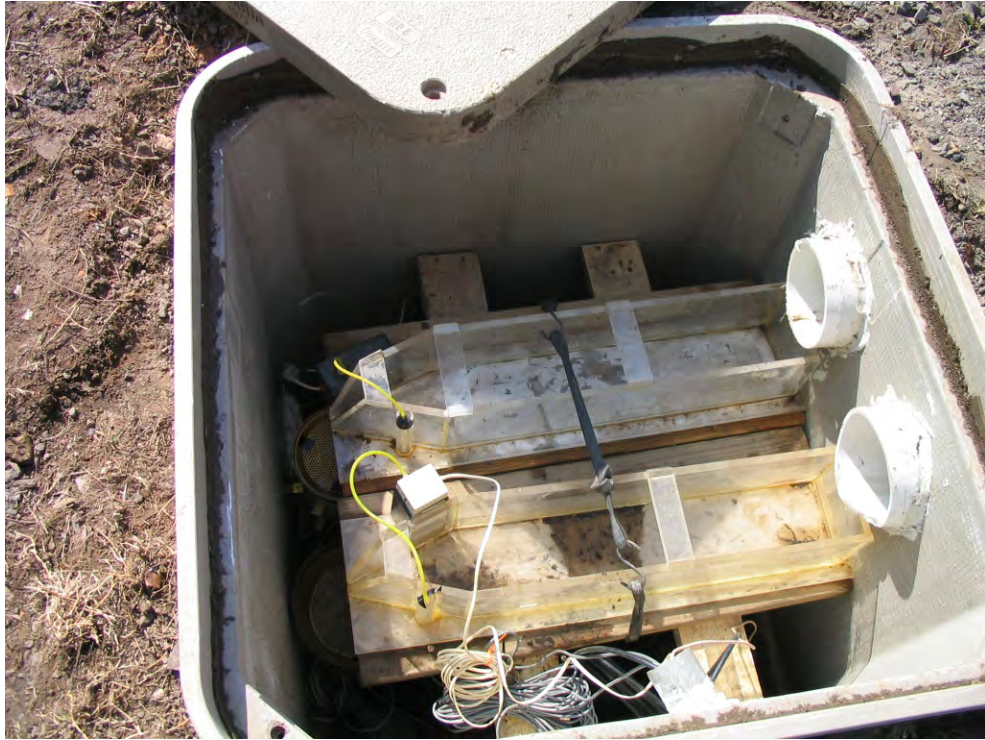
Figure 3.72 Flumes and tipping bucket flowing meters housed in a fiber glass box.
