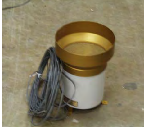
Figure 3.41 TR-525USW rainfall sensor.
