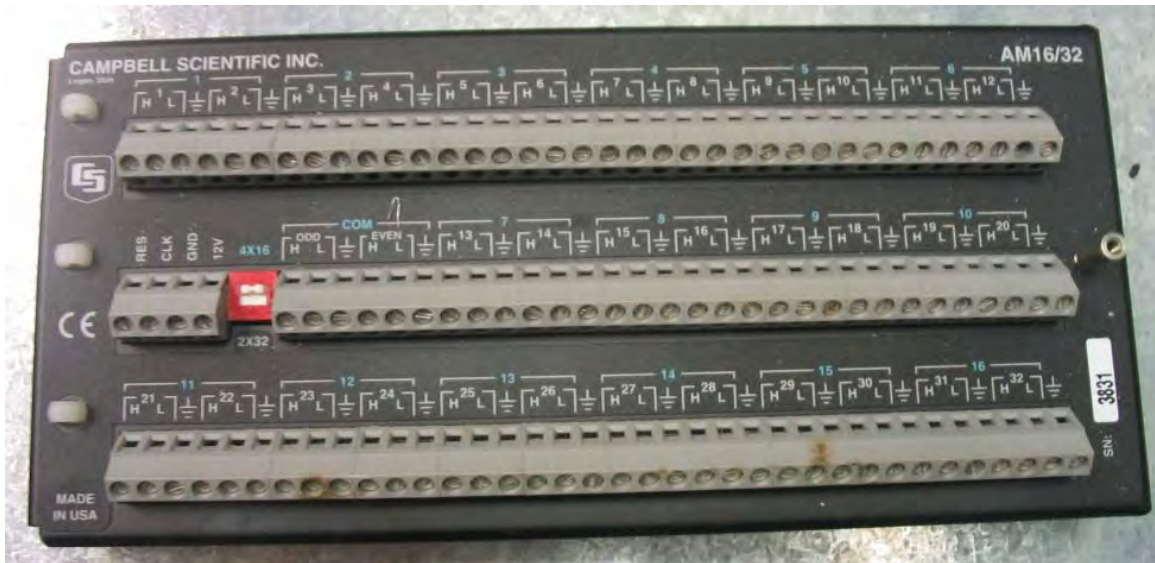
Figure 3.27 Campbell Scientific, Inc, model AM16/32 Multiplexer.
