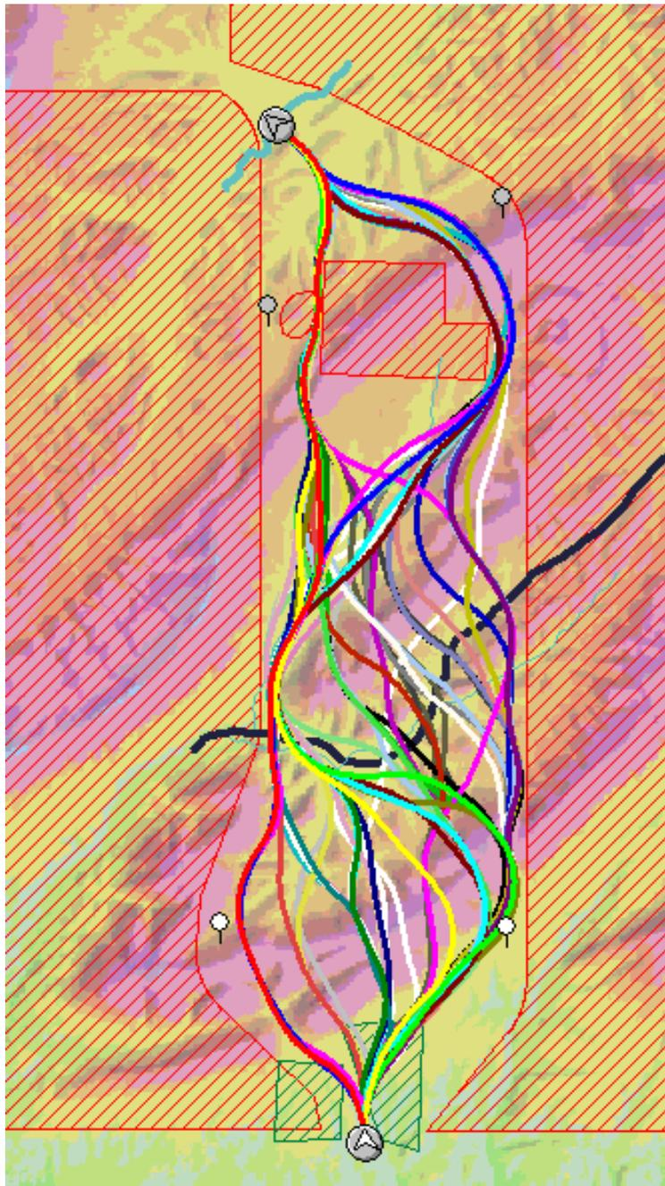
Using Quantm Integrator, the Department’s planners were able to (1) conduct a local review of Quantm Pathfinder generated alignments to assess qualitative and quantitative properties of each option, (2) generate and output earthworks and costs reports, (3) display alignments on DTM, (4) generate aerial photographs, (5) generate cross section views and vertical profile views in a CAD program. Figure 3 shows Alternative A and B alignments near the end of the selection process.
