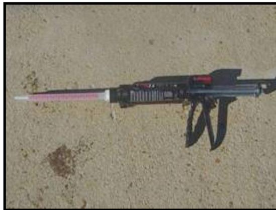
**Figure 7.10 Epoxy Dispensing Tool**
