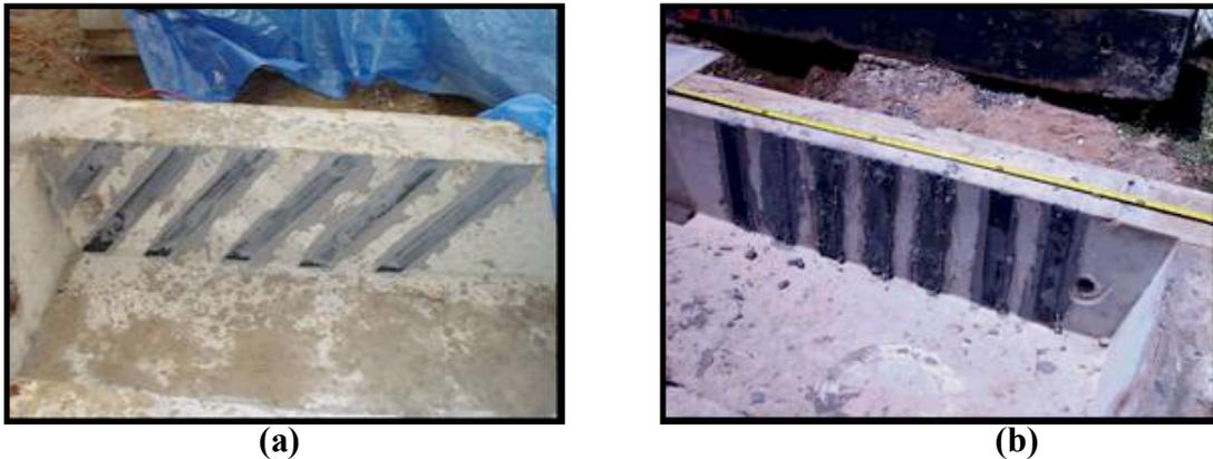
**Figure 7.6: CFRP Vertical and Diagonal Retrofitted Beams**
