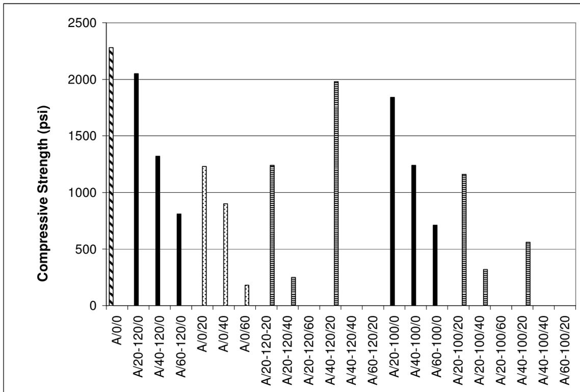
Three-day compressive strength values are listed in Table 4.5 except for the A/40-100/20 mixture. The six compressive strengths were not recorded for A/40-11/20. The highest three-day compressive strength was the control mixture (A/0/0) with a compressive strength of 5290 psi. The second highest three-day compressive strengths were recorded for A/20-120/0, A/0/20, A/20-120/20, and A/20-100/0 with compressive strengths ranging from 4260 to 4020 psi respectively. The next grouping
