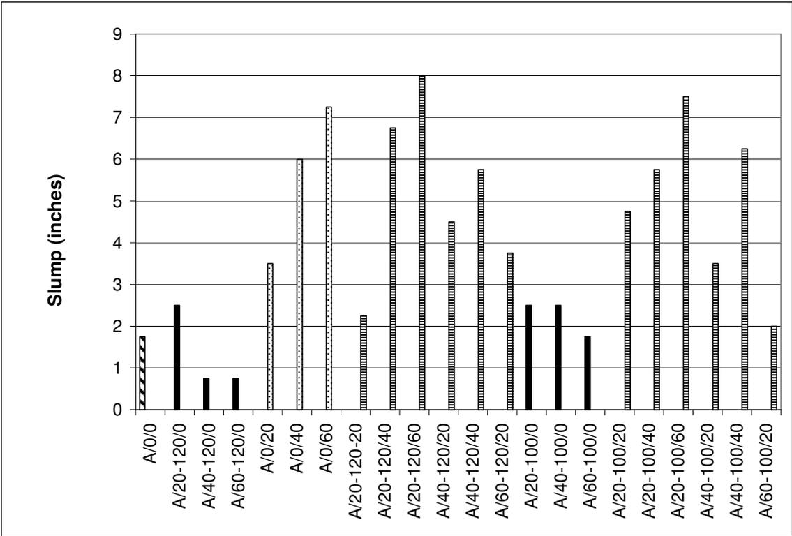
Trends from this study were consistent with the previous research that suggests that the addition of FA increases workability through the small, spherical particles
