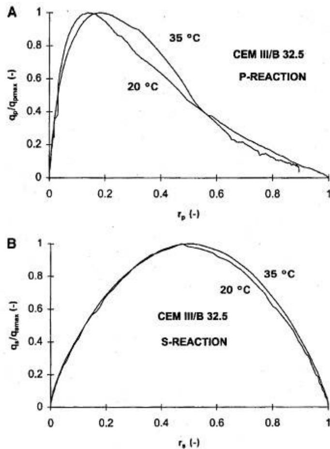
The reaction curves show that portland cement mixtures gain heat more rapidly than GGBFS. The heat gain curves also show slag cement heat gain begins later than the portland cement, explaining the slower heat of hydration and the increase in set times for mixtures containing GGBFS (Schutter, 1999).
