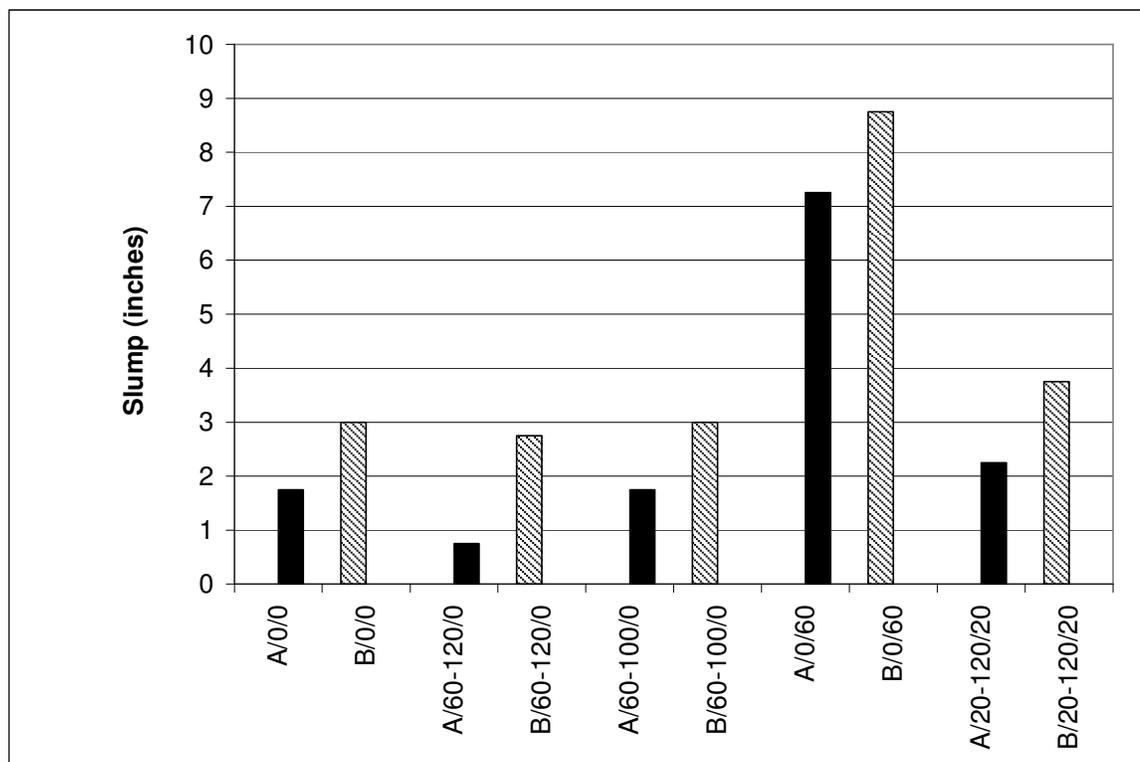
The 5.5 in. to 5.75 in. increase in slump over the control mixture shown by both batches with 60% FA replacements was consistent with literature. Fly ash particles are small and spherical which helps lubricate the mixture. The ternary
