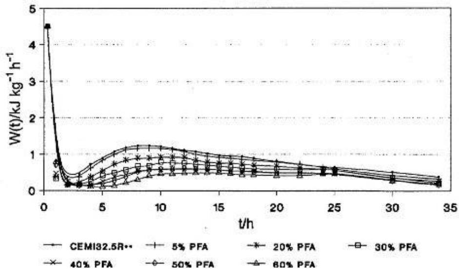
Schutter described the hydration of slag-cement concrete as a two fold reaction of the portland cement and the slag that can be superimposed onto one heat curve and estimate the slag-cement heat curve. An adiabatic hydration test, where heat is not lost or gained from the system (Agnes, 2000), measured the heat production rate as a
