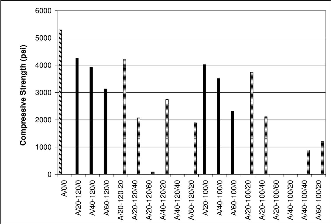
At seven days of age, the A/20/0, A/20/60, A/40/40, and A/60/20 mixtures had not statistically different compressive strengths between the GR 100 and GR 120 GGBFS mixtures. The A/60/0, A/20/20, A/20/40, and A/40/20 mixtures saw a 11%,
