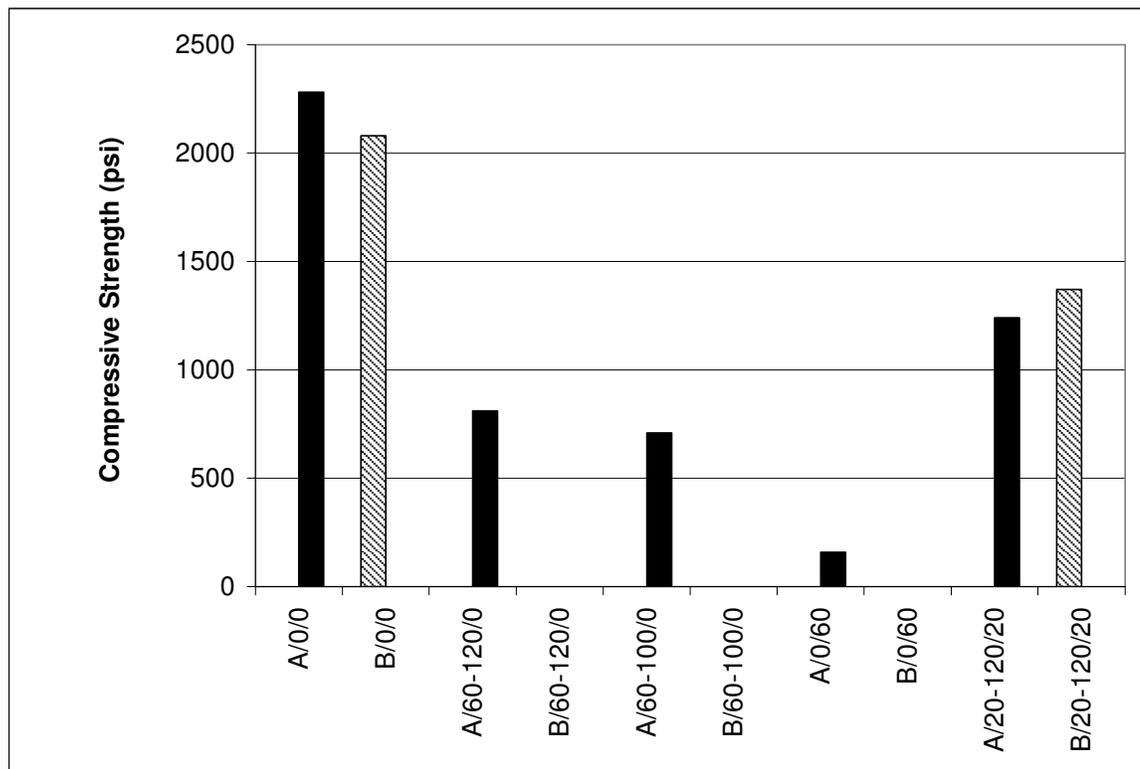
Statistical analysis on the three-day compressive strengths showed that for each replacement rate the cement A and cement B mixtures had not statistically different compressive strengths (i.e. the cements were interchangeable for strength gain at 3 days). The control mixtures (A/0/0 and B/0/0) also had not statistically
