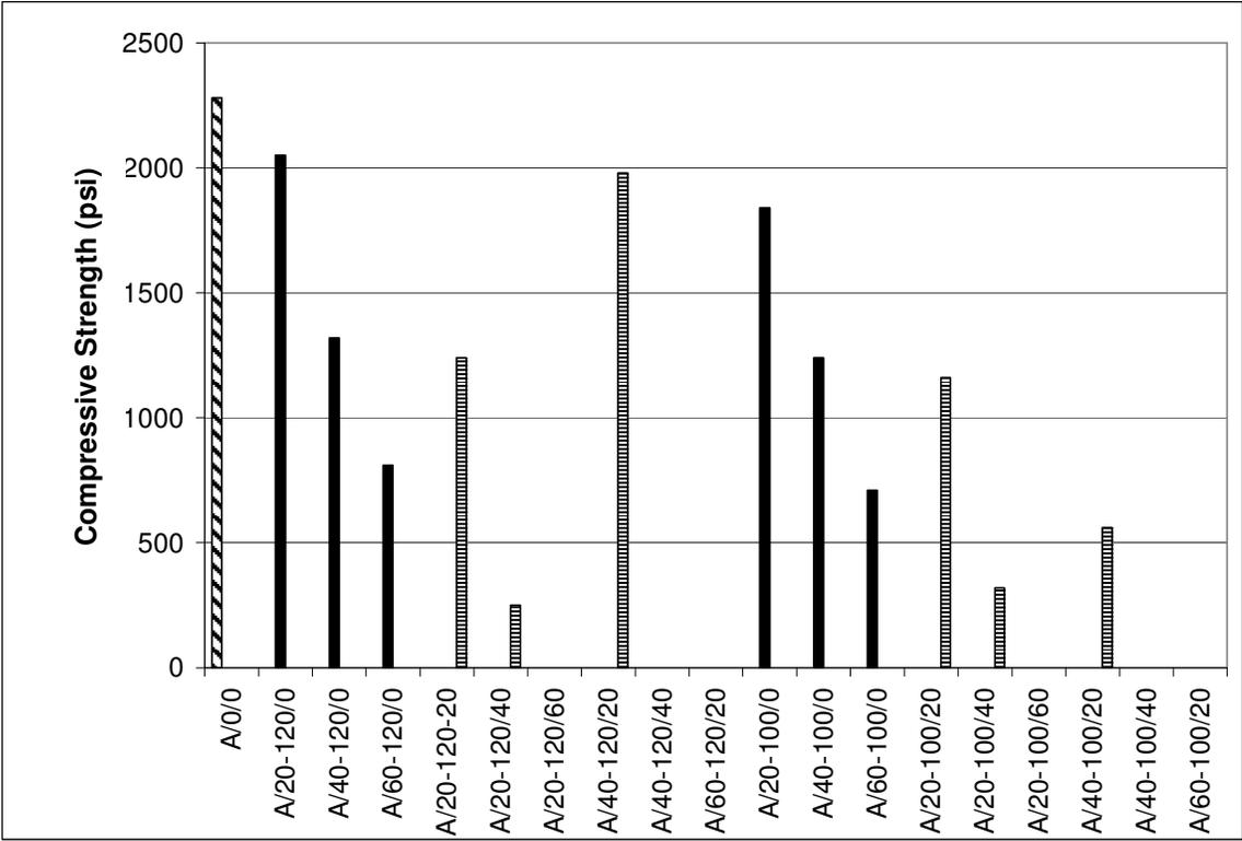
At three days of age, mixtures that had not statistically different compressive strengths were A/20/0, A/20/40, A/20/60, A/40/40, and A/60/20. The A/40/0, A/60/0, and A/20/20 mixtures had an average of 14% less three-day compressive strength
