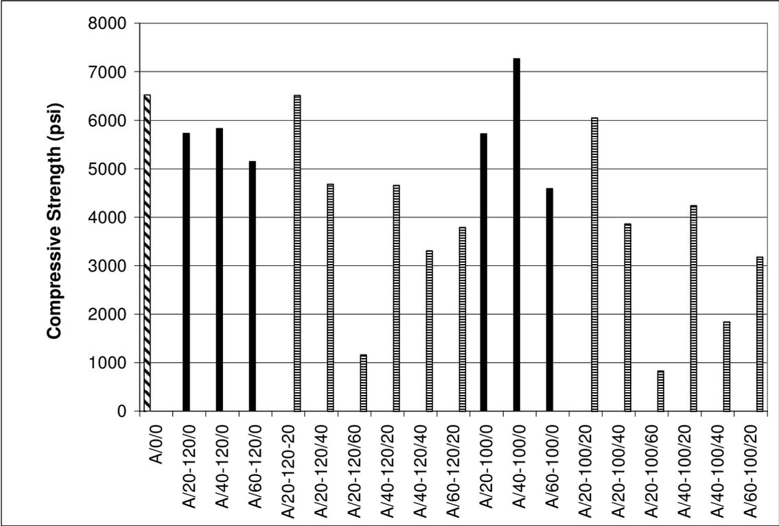
The mixtures that had not statistically different twenty-eight day strengths whether they were made with GR 100 or GR 120 GGBFS were A/20/0, A/20/20, A/20/60, and A/40/40. Four of the remaining five mixtures had greater twenty-eight day compressive strength when made with GR 100 GGBFS. These mixtures were A/40/0, A/60/0, A/20/20, A/40/20, and A/60/20. The trends in twenty-eight day compressive strength data and Chart 4.32 were observed to be as follows:
