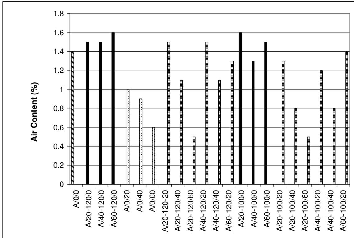
Reduction in air content with increases in FA content correlates with the increased workability observed in the FA mixtures. As discussed in the literature review section, both events could be directly related to the spherical shape of the FA particles. The smooth, round particles would allow entrapped air to easily escape; unlike the crushed and jagged particles of the cement and GGBFS that would entrap more air.
