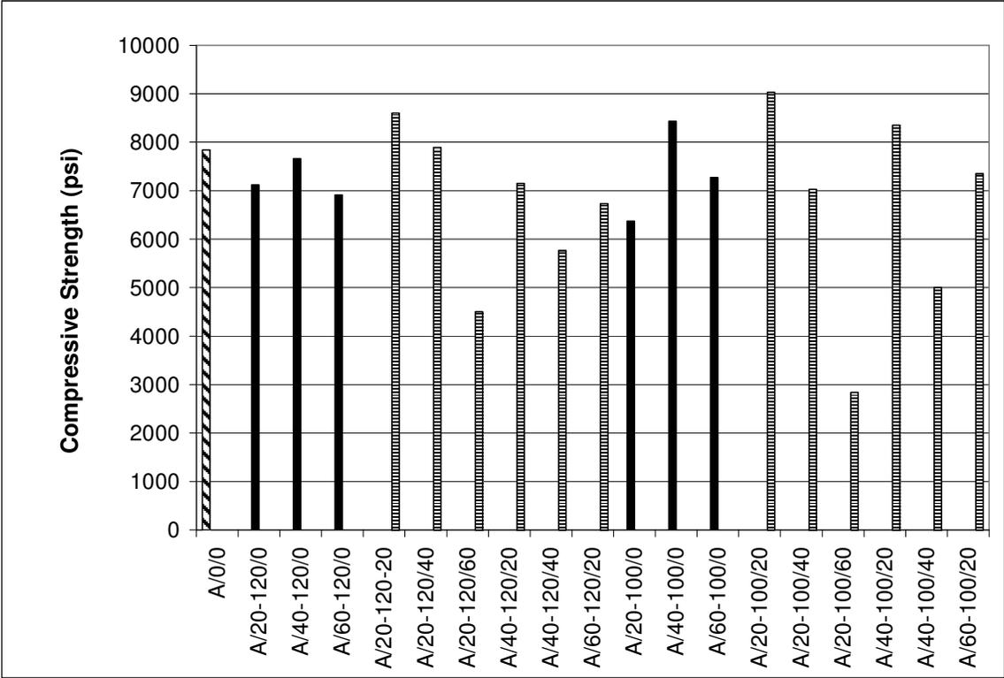
Not statistically different mixtures in ninety-day compressive strength between GR 100 GGBFS and GR 120 GGBFS were: A/20/0, A/40/0, A/60/0, A/20/20, A/20/40, and A/40/40. The A/40/20 and A/60/20 mixtures were decreased by 11% when made with GR 120 GGBFS. The A/20/60 mixture had a 15% decrease in ninety-day compressive strength when made with GR 100 GGBFS. The 90 day compressive strength trends observed were as follows from the data and Chart 4.33:
