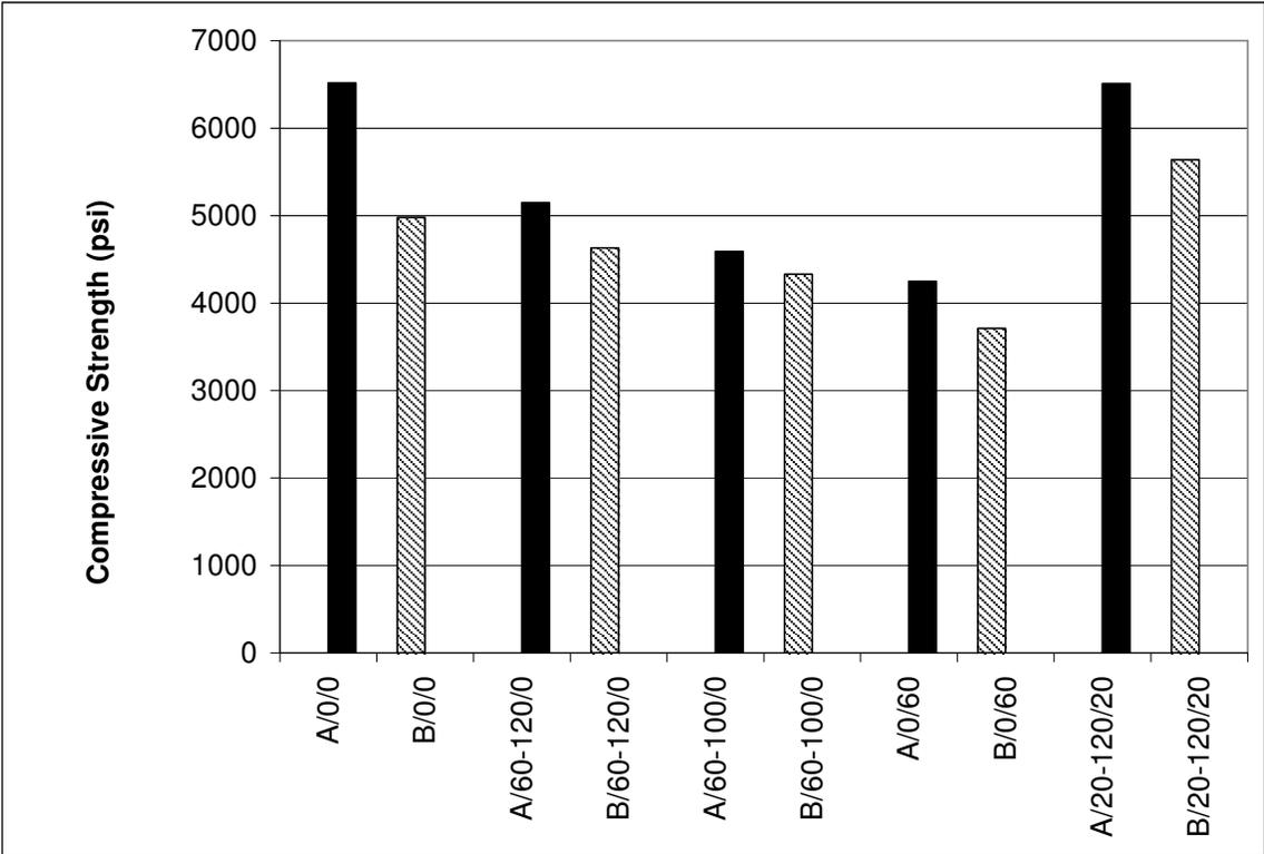
Twenty-eight day compressive strength results showed that the ternary mixtures gained more strength than the corresponding control mixture. The cement A ternary mixture, A/20-120/20, had the greatest twenty-eight day compressive strength at 8600 psi. The cement B ternary mixture, B/20-120/20, had the greatest twenty-eight day compressive strength of the cement B mixtures with 7290 psi but was 15% less than the A/20-120/0 mixture. The trends in the data and Chart 4.8 were observed as follows:
