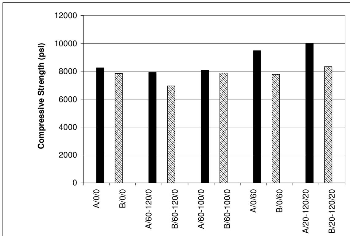
The cement study suggested that the two sources of cement did not create the same compressive strengths with the same replacement mixtures. They, however, had similar trends in mixtures with similar replacements of cement. The replacements of
