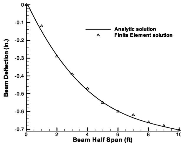
**Figure 3. Beam deflection result comparison.**
