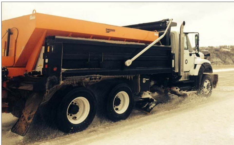
Figure 1: New AHTD Belly Plow
