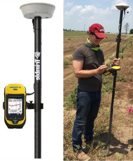
Figure 2. 11: Trimble GPS with external antenna.
