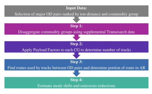
FIGURE 0-1. PROCESS FOR ESTIMATING IMPACTS ON THE TRUCKING INDUSTRY
