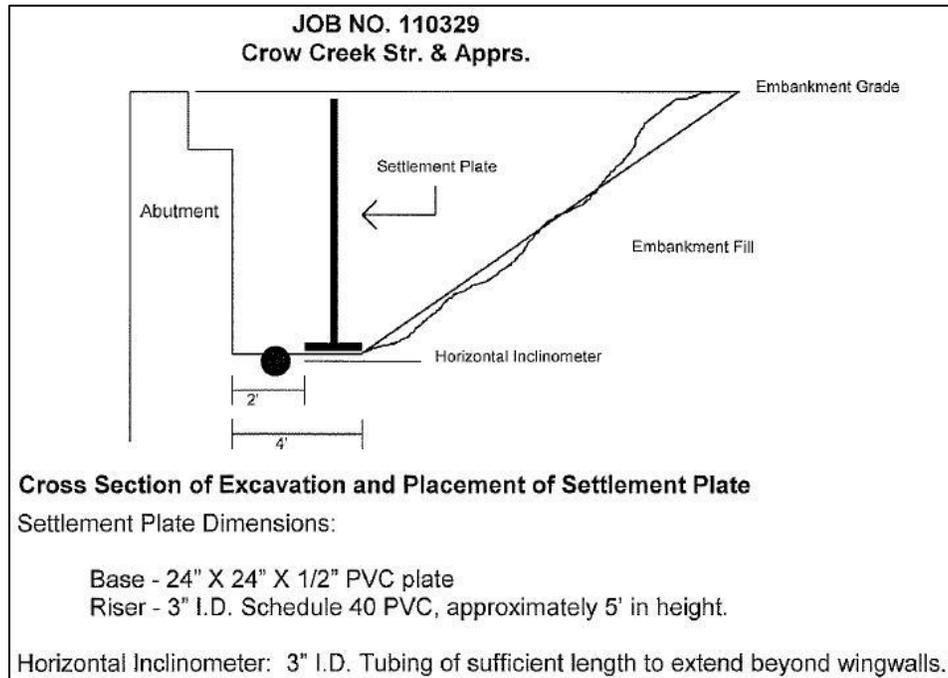
**Figure 21. Crow Creek general settlement plates and horizontal inclinometer locations.**
