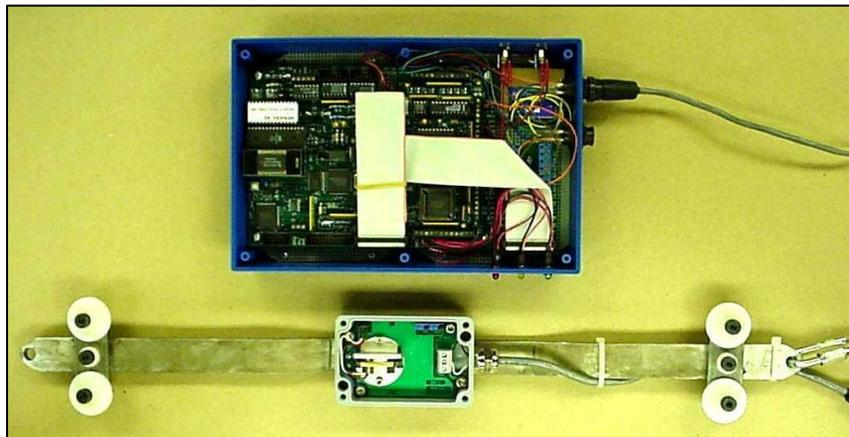
**Figure 5. Horizontal inclinometer setup, data logger (upper) and inclinometer sensor (lower).**
