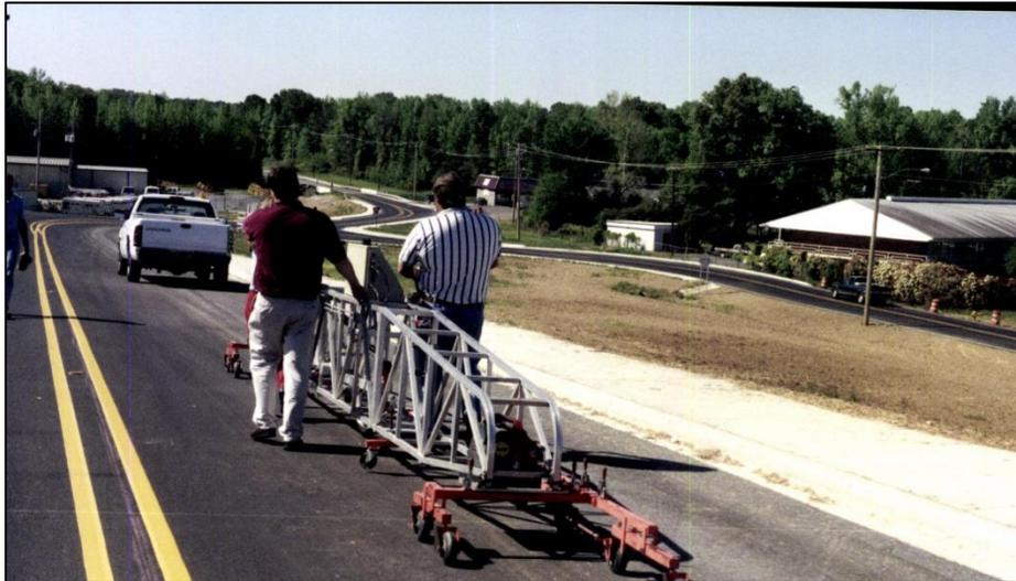
Figure 27. California profilograph at Chicot Road Bridge.
