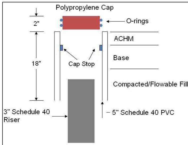
Figure 3. Access tube components.
