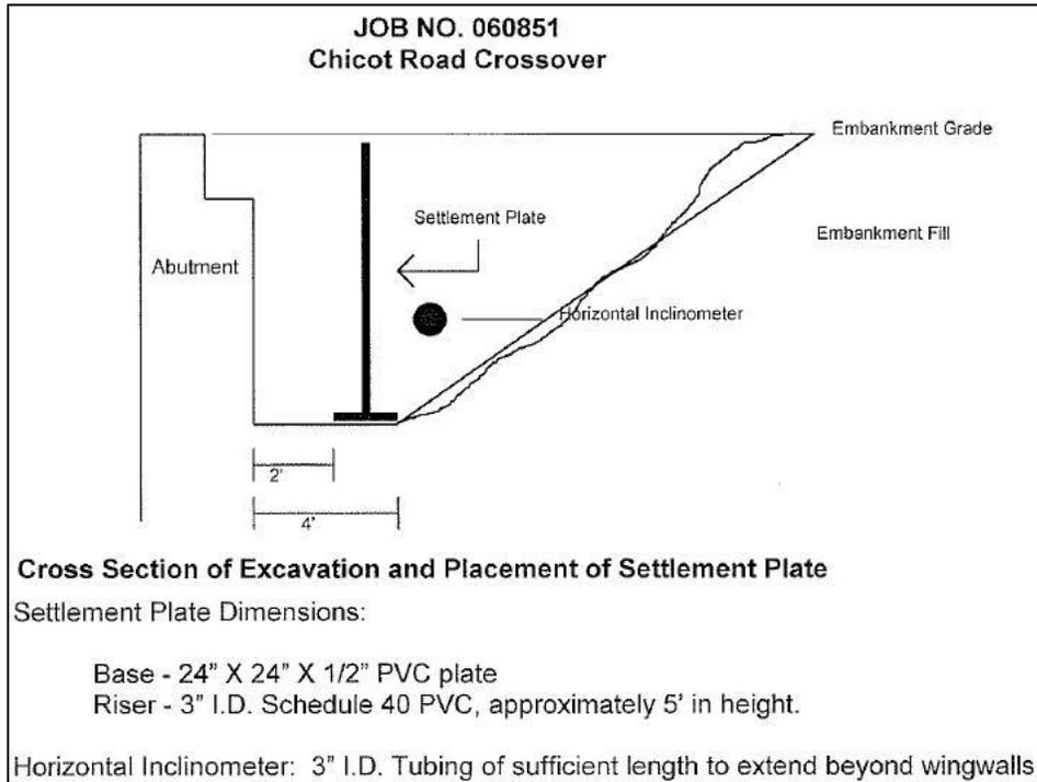
Figure 15. Chicot Road general settlement plates and horizontal inclinometer locations.
